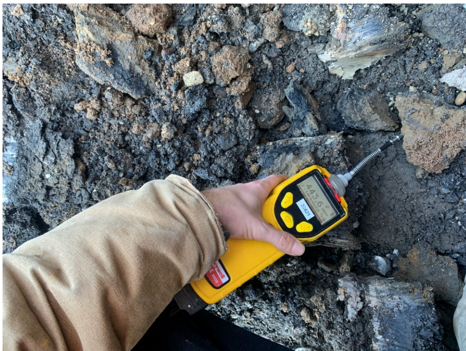
Photograph No. 3: Representative photo of soil screening around concrete encasement on 2/5/24.
