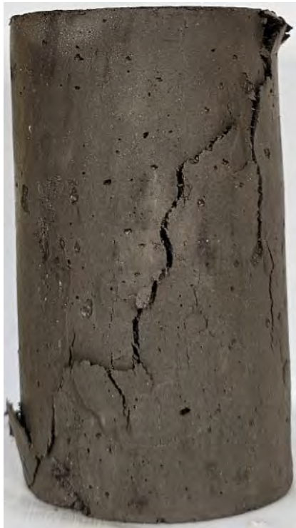
Failure Photograph of Specimen
