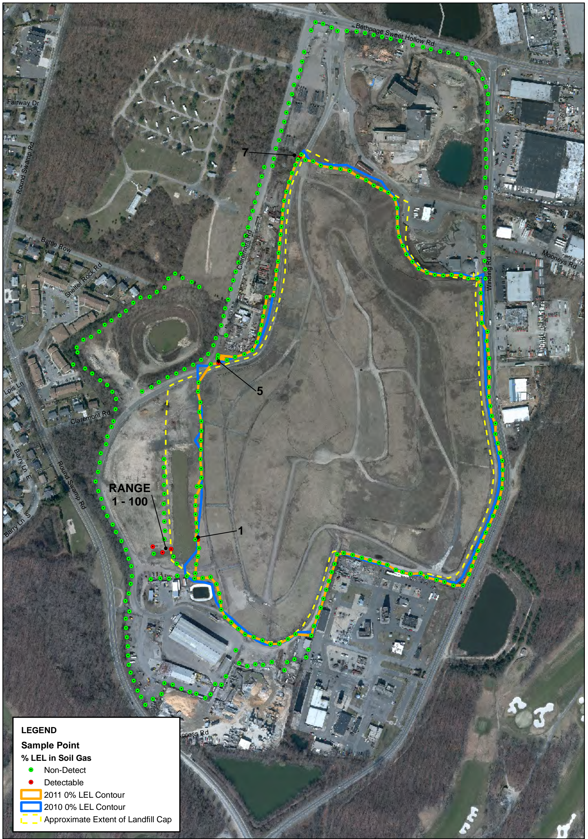
FIGURE 3.3 2011 ANNUAL ZERO GAS MIGRATION LIMITATION SURVEY TOWN OF OYSTER BAY SOLID WASTE DISPOSAL COMPLEX OLD BETHPAGE, NEW YORK
