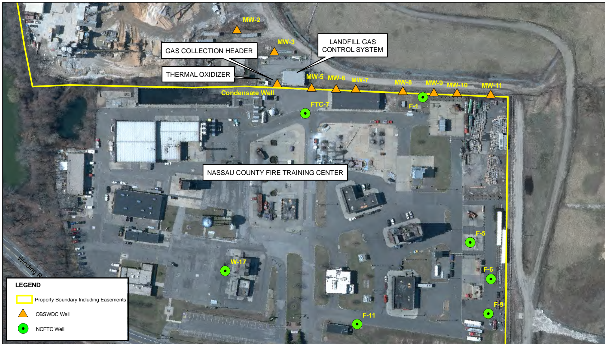
FIGURE 3.2 LANDFILL GAS HEADER AND WELLS ADJOINING NASSAU COUNTY FIRE TRAINING CENTER
