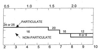
Duct Diameters Downstream From Flow Disturbance
