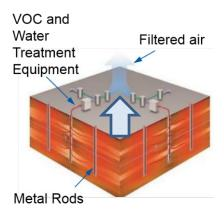
arrow on the illustration). Also, an engineered cover with a dedicated vapor recovery system was installed over the treatment areas to ensure vapors do not escape from the surface.
