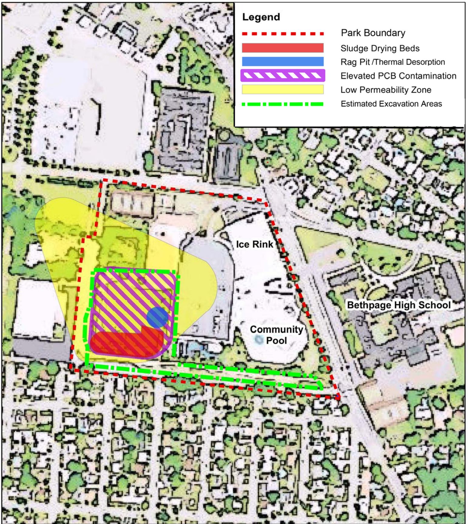
ESTIMATED EXCAVATION AND THERMAL DESORPTION AREAS New York State Department of Environmental Conservation Grumman Aerospace-Bethpage Facility Bethpage, Nassau County, New York
