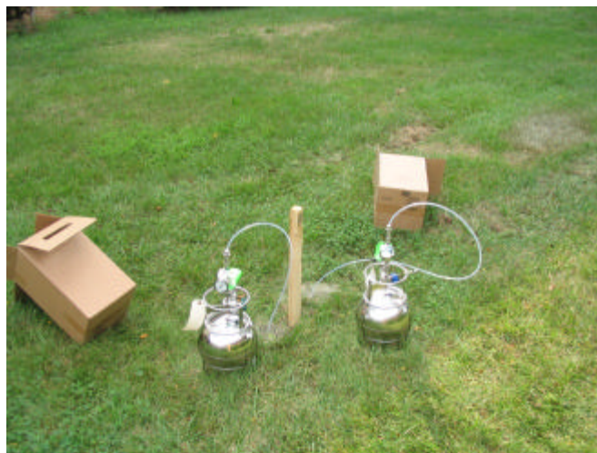
Sampling of Shallow and Deep Soil Vapor Points
