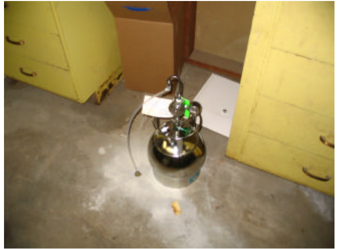
Sub-Slab Vapor Sample
