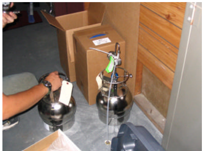
Final Set-up of Sub-Slab Vapor Sample
