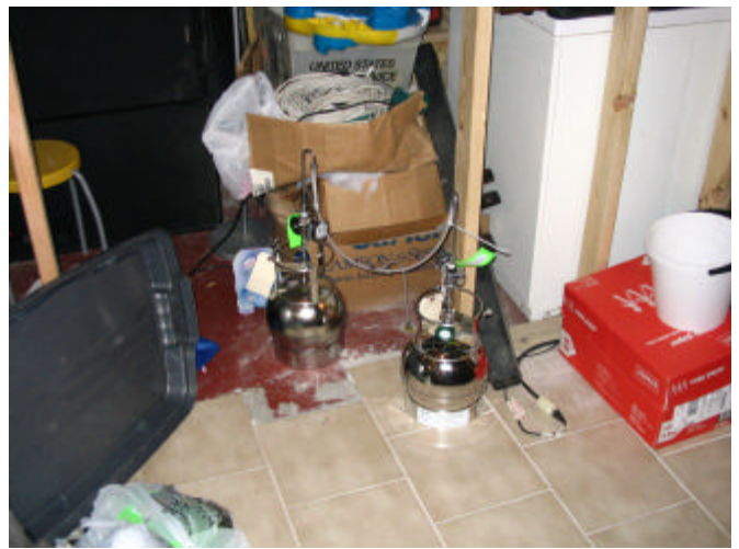
Duplicate Sub-Slab Sample Collection
