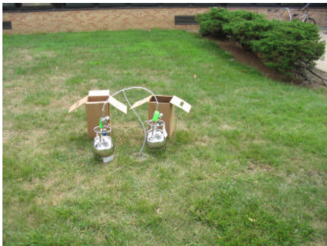
Sampling of Soil Vapor Point and Duplicate Sample
