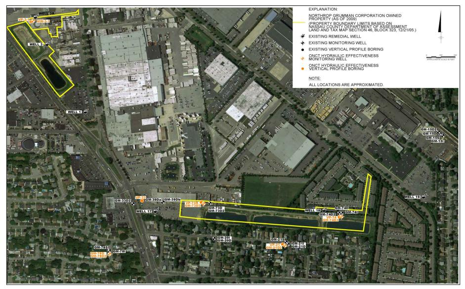
SITE PLAN SHOWING MONITORING WELLS AND VERTICAL PROFILE BORINGS
