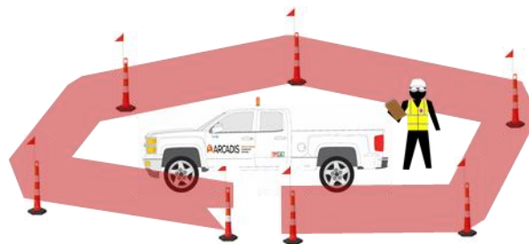
Scenario #2: Long Term (>8 Hours) Channelizing Cones with Flags and Safety Fencing
