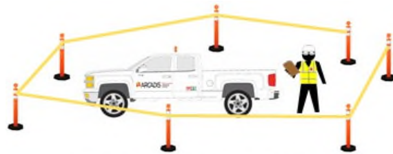
Intermediate Term (1-8 Hours) Channelizing Cones with Caution Tape
