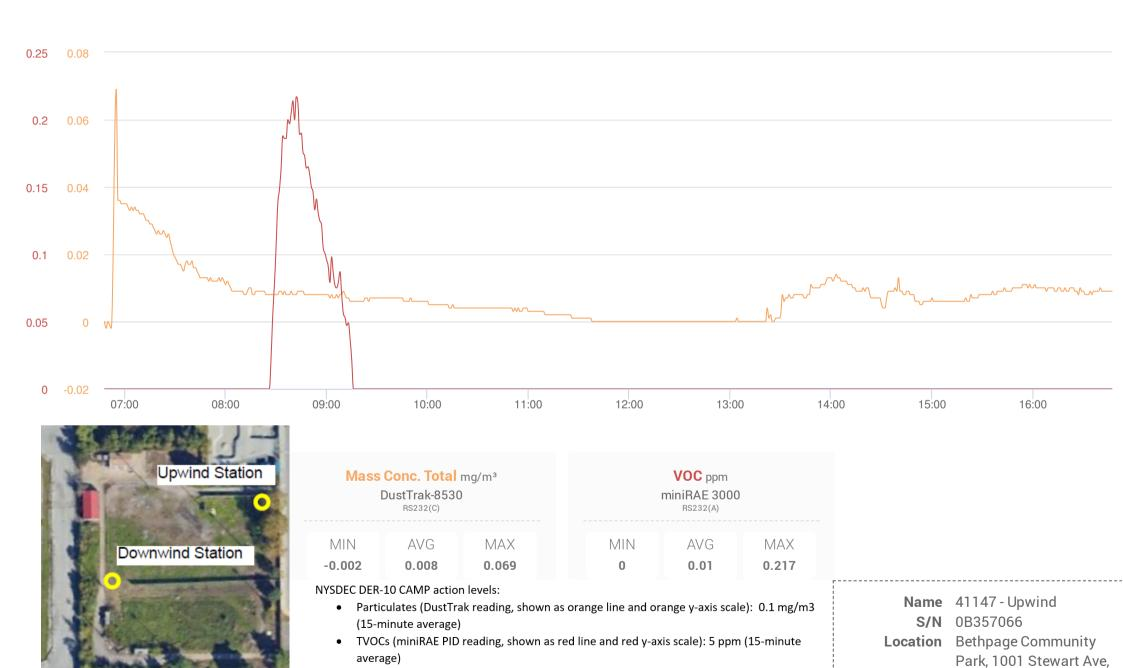
Short-term peaks of DustTrak and miniRAE readings are common during instrument setup at the beginning of the workday, and during manual calibration/detection checks throughout the day.
