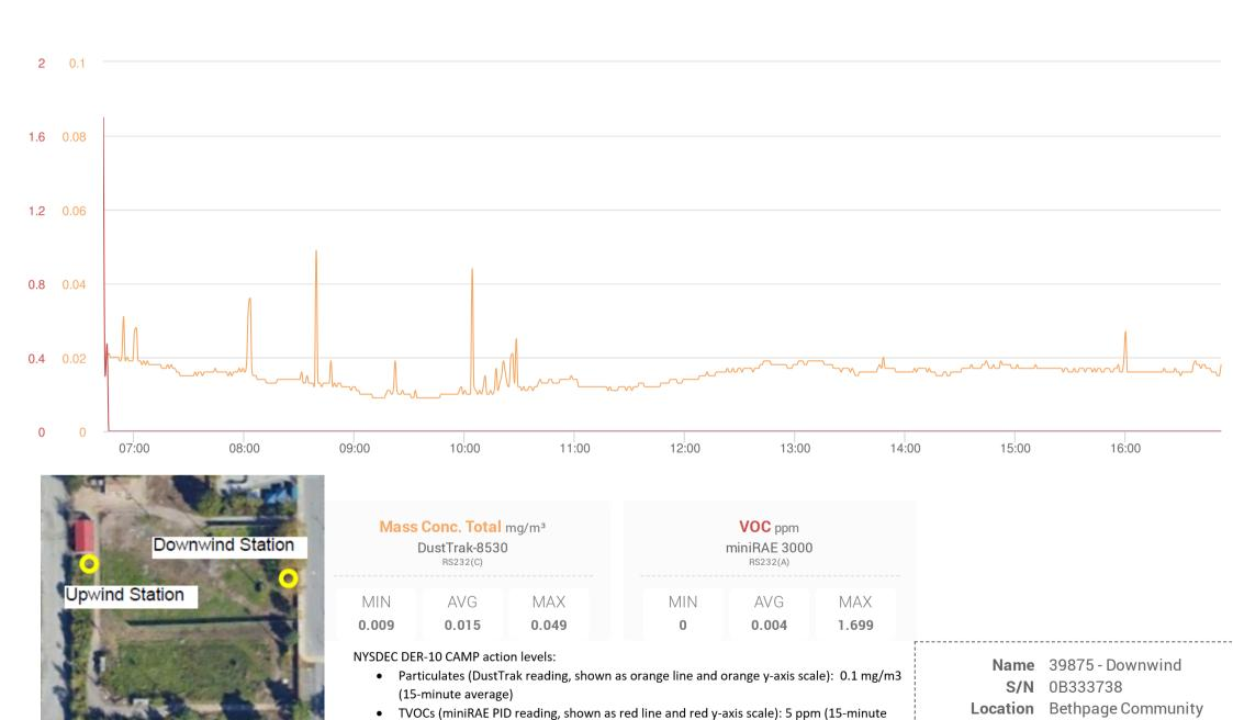
Short-term peaks of DustTrak and miniRAE readings are common during instrument setup at the
