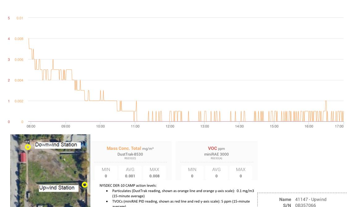
Short-term peaks of DustTrak and miniRAE readings are common during instrument setup at the
