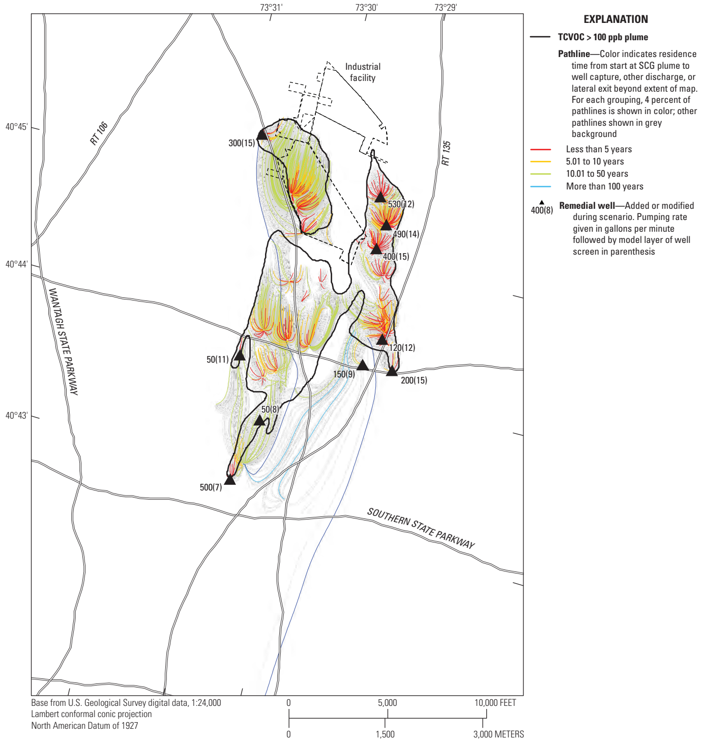
Figure 22. Map showing scenario 4 pumping wells, the total chlorinated volatile organic compound (TCVOC) greater than (>) 100-part-per-billion (ppb) plume shell (HDR, 2019), and particle pathlines starting at the plume shell, southeastern Nassau County, New York. A high-resolution version of this figure is available for download at https://doi.org/10.3133/sir20205090 .
