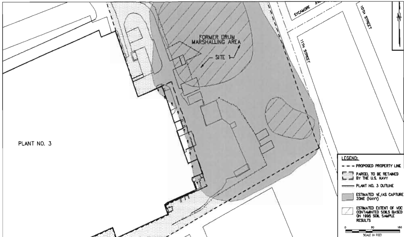
Figure 5 Area Requiring Treatment of Soil for VOCs
