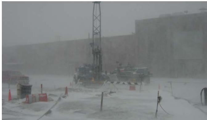
Soil samples are collected using the hollow stem auger drilling method.
