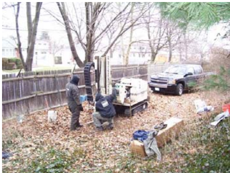
Soil gas sampling along the eastern border of NWIRP in January 2008. Sampling indicated elevated levels of volatile chemicals at the facility boundary.
