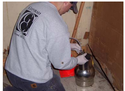
Indoor air sampling was conducted in January 2009 in homes along 11 th Street. Results indicate elevated levels of TCE in the indoor basement air of several of the homes sampled.
