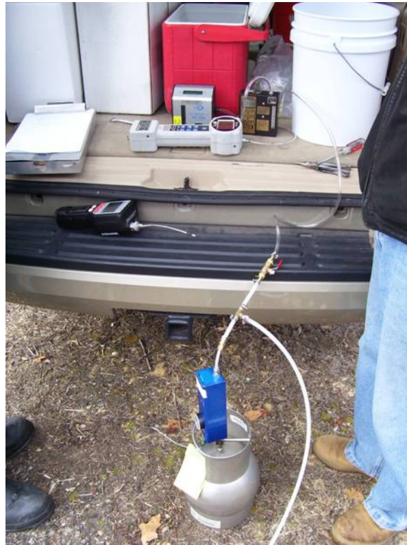
Photo 9: Summa canister and purge pump.
