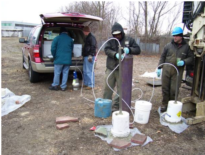
Photo 12: DPT rig and sample points, East of Site 1.
