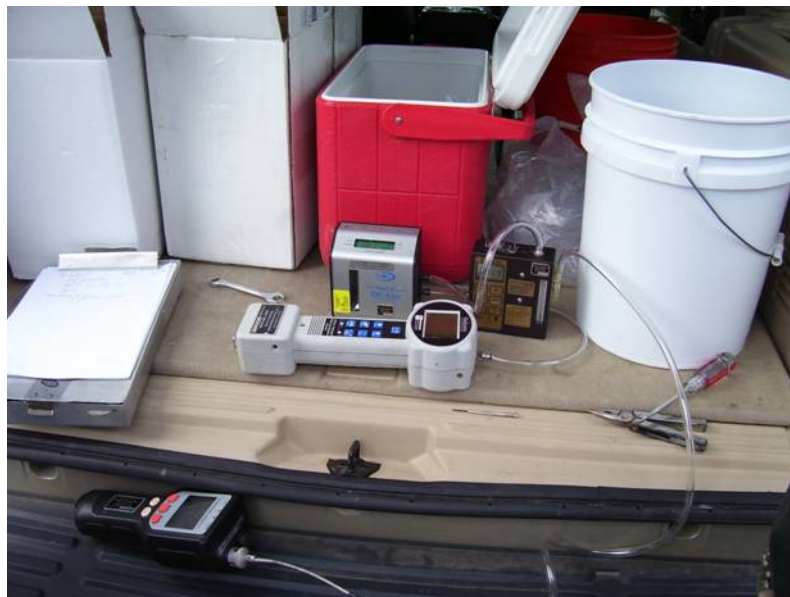
Photo 10: Purge pump and helium detector.
