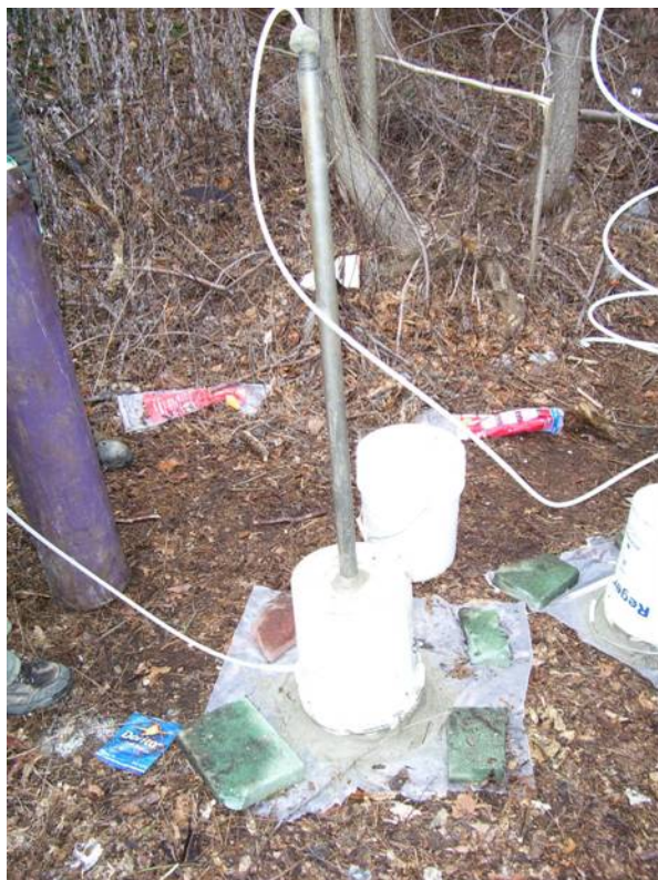
Photo 7: Probe tubing, helium tank over sample point.
