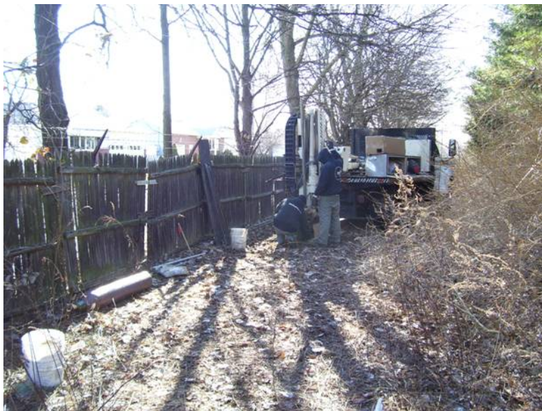
Photo 6: DPT rig, East of Site 1
