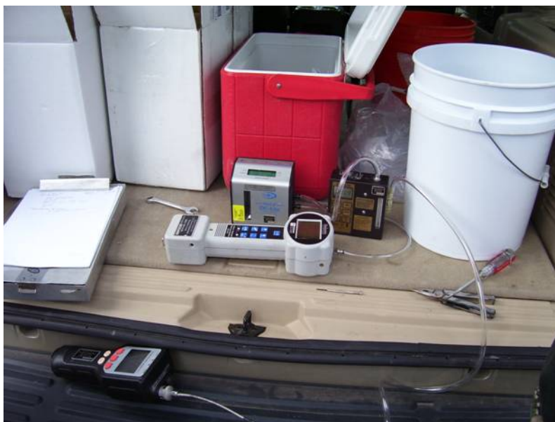
Photo 10: Purge pump and helium detector.
