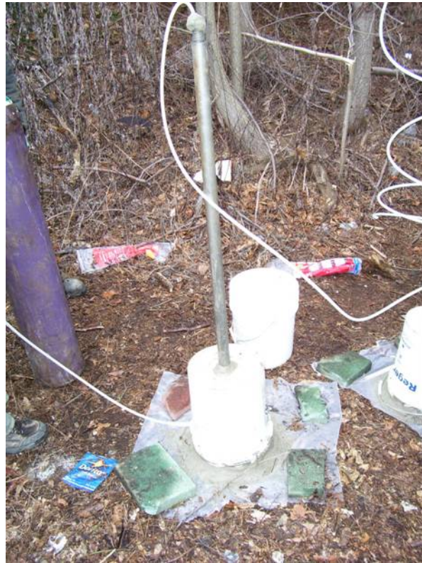
Photo 7: Probe tubing, helium tank over sample point.
