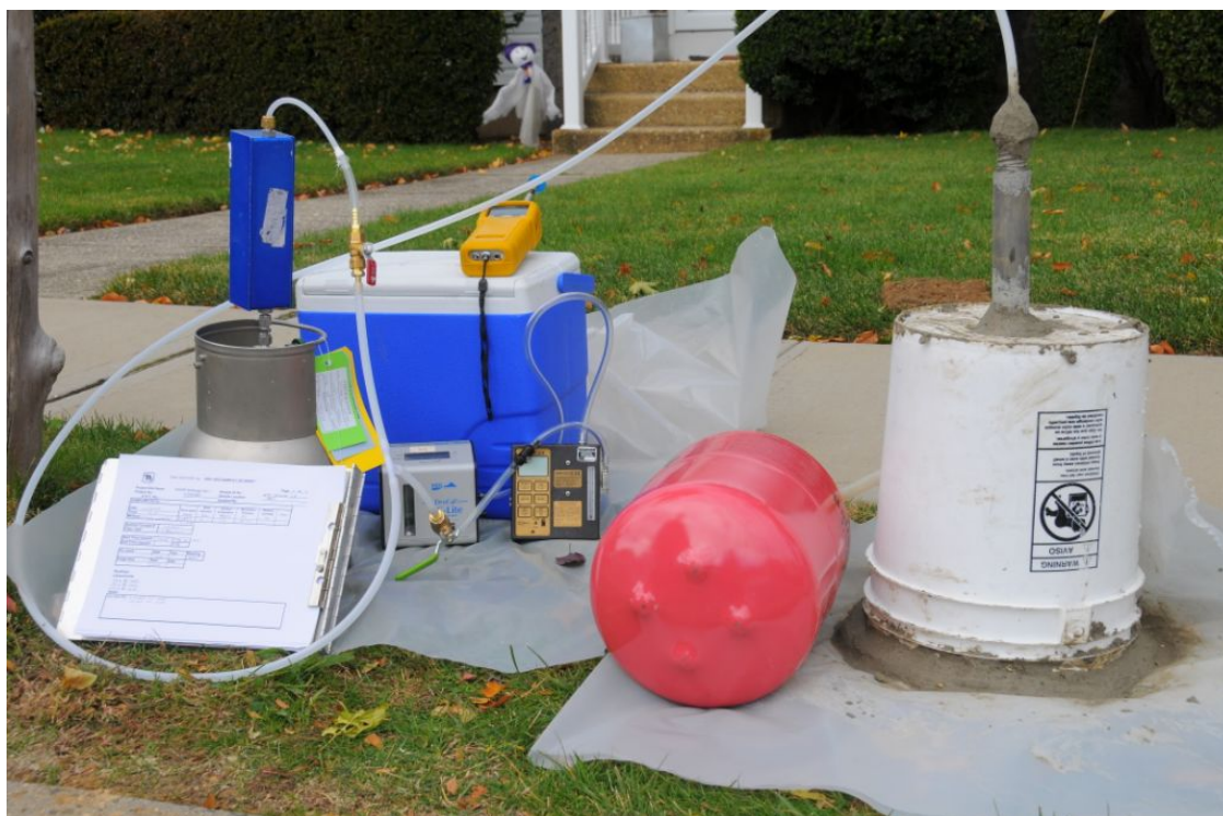
Photo 2: BPSI-SG2008 showing typical soil gas sampling setup.
