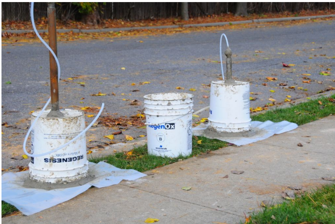
Photo 5: Close up of BPSI-SG2001 showing soil gas points post-sampling.
