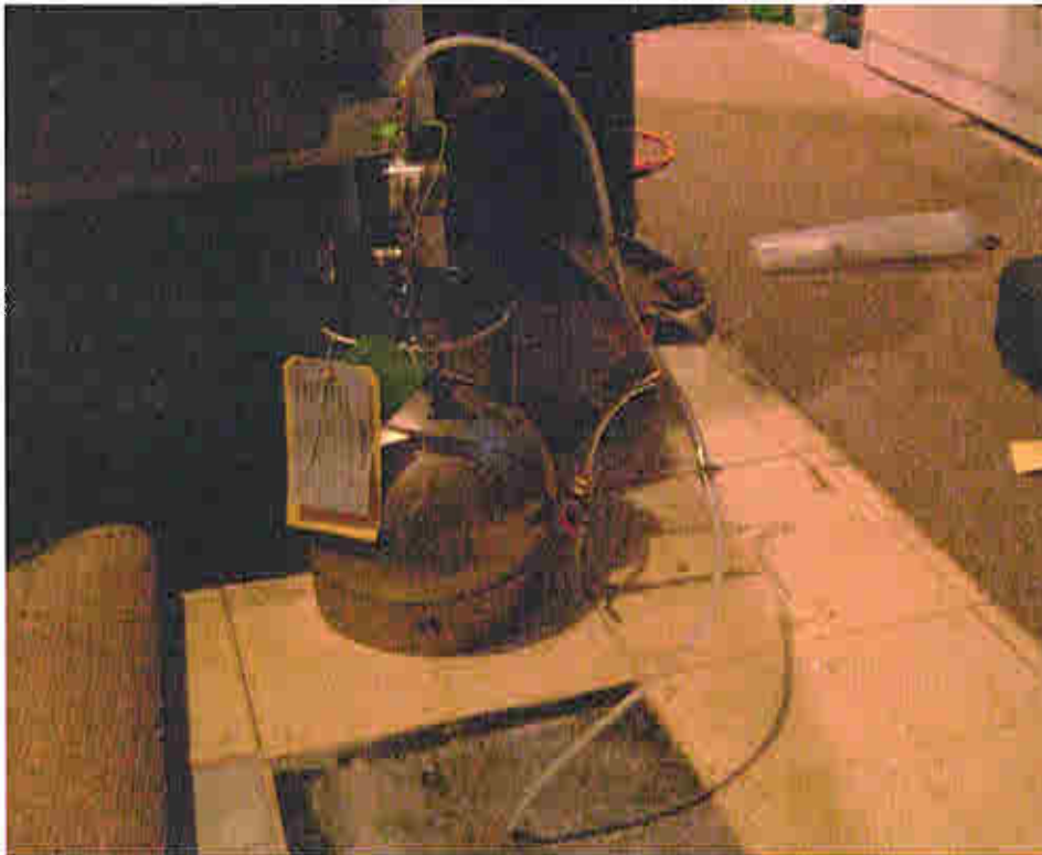
Photo 22: Sub-slab sample location at Home #6.
