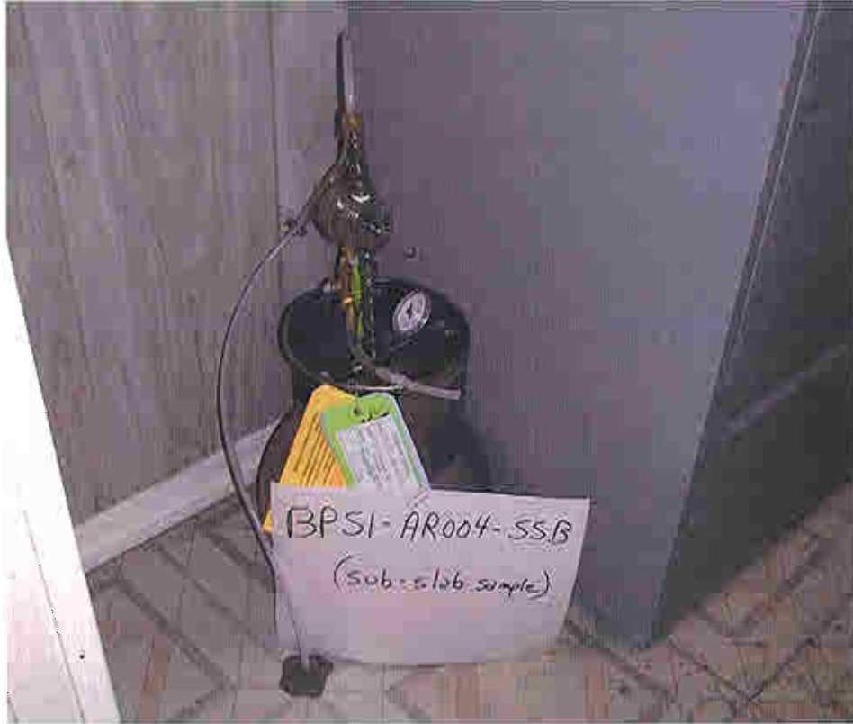
Photo 13: Sub-slab sample location at Home #4.
