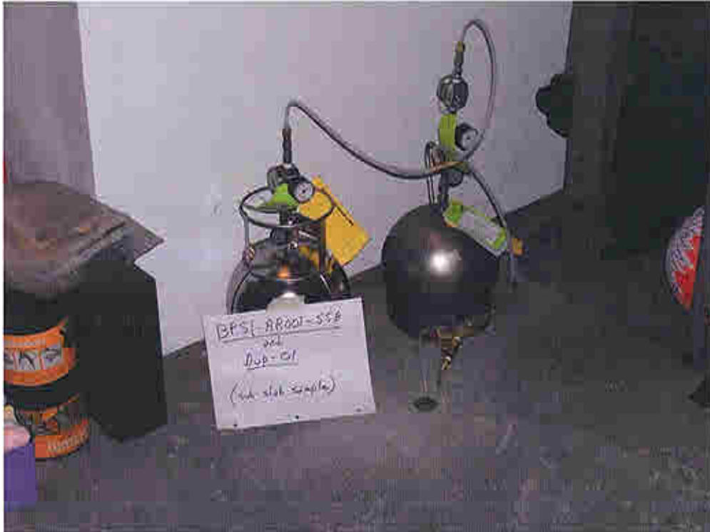
Photo 1: Sub-slab sample location with duplicate from Home #1.
