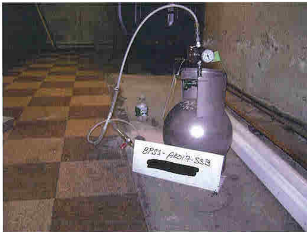
Photo 59: Sub-slab sample location at Home #17.
