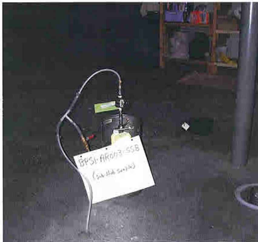
Photo 8: Sub-slab sample location at Home #3.
