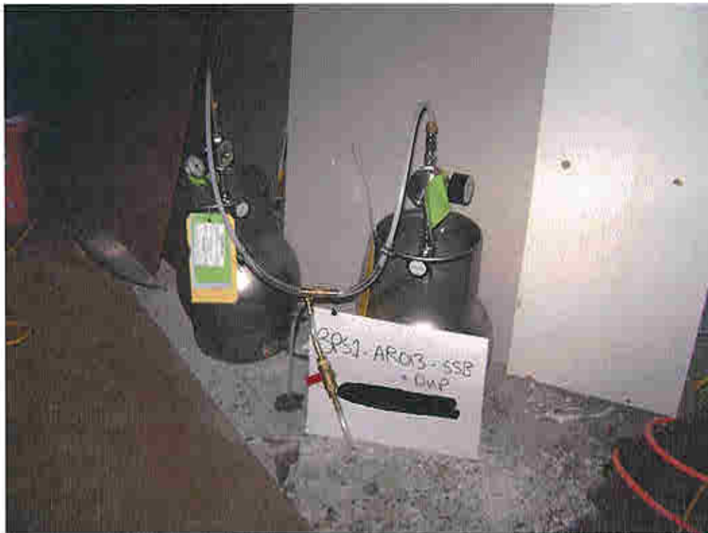
Photo 46: Sub-slab sample with duplicate collected from Home #13.
