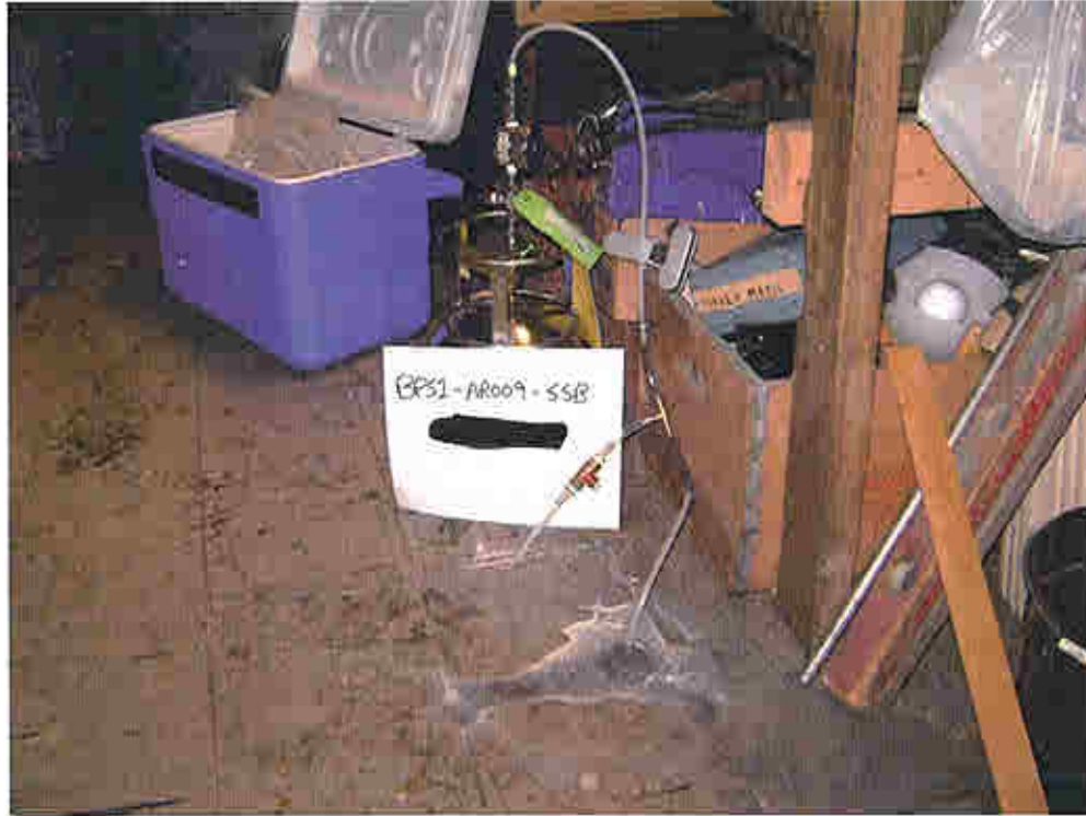
Photo 33: Sub-slab sample at Home #9.
