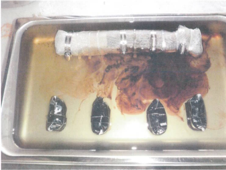
Photo 14: The cylinder has been returned for the second soak in VertecBio Gold #4, the cylinder is draining. Oil drained from the cylinder following the first soak. .
