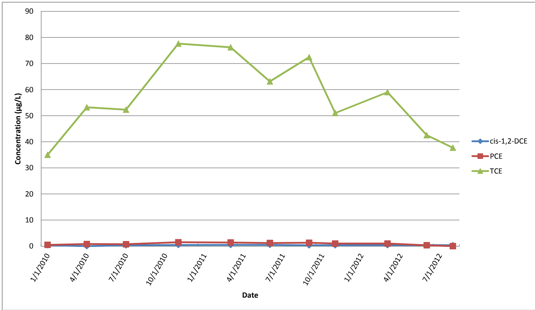
Figure 10 GM-38 Area Groundwater Remediation Naval Weapons Industrial Reserve Plant - Bethpage, NY Groundwater Concentration Trends of Select VOCs RW3-MW1
