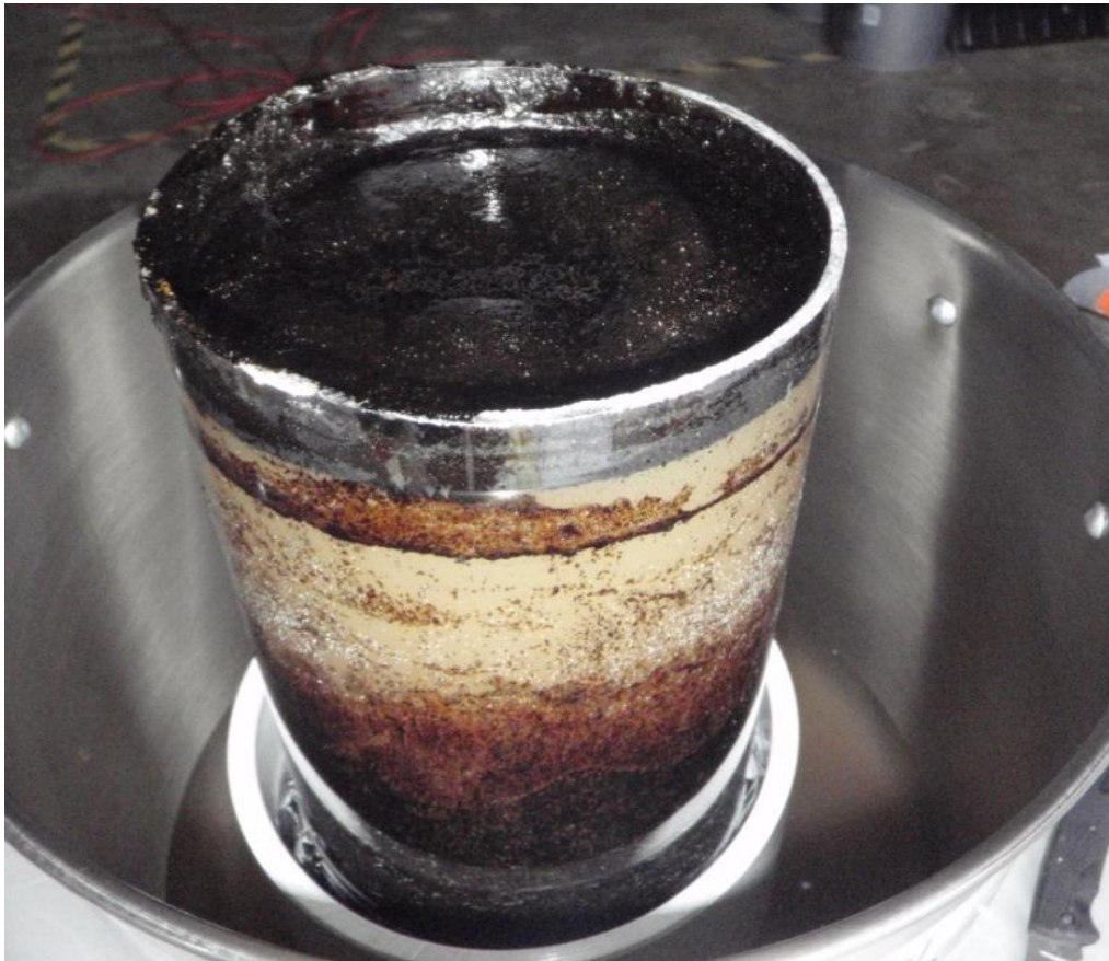
Photo 2 - View of film of product that formed on top of the hot water in Test TN-3003.
