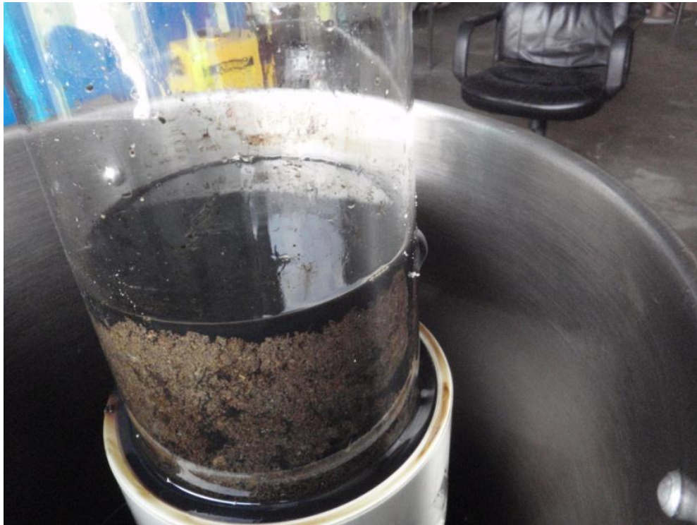
Photo 6 - View of product seeping out of side holes in the cylinder in Test TN-3004.
