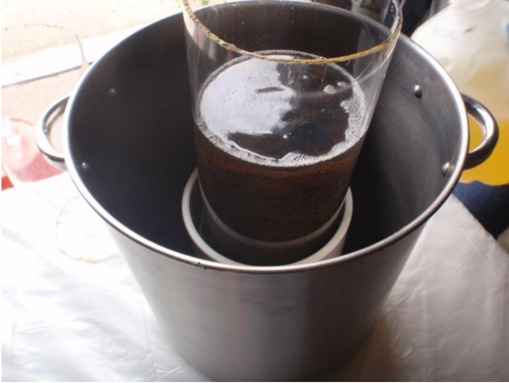
Photo 5 - Side view of column of unsaturated soil after diesel was added in Test TN-3003.
