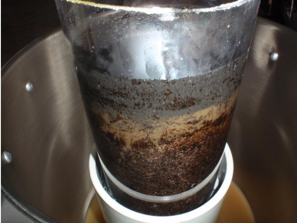
Photo 2 - View of film of product that formed on top of the hot water in Test TN-3003.
