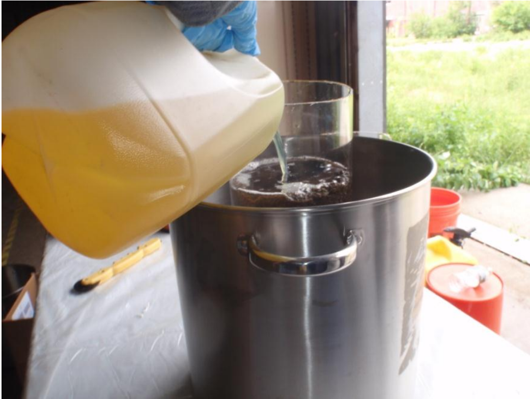
Photo 3 - Addition of diesel to unsaturated soil in Test TN-3003
