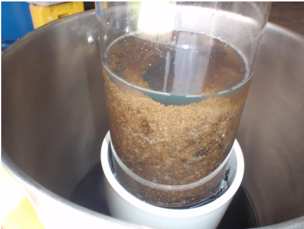
Photo 4 - Side view of column of unsaturated soil after Vertec was added in Test TN-3003.
