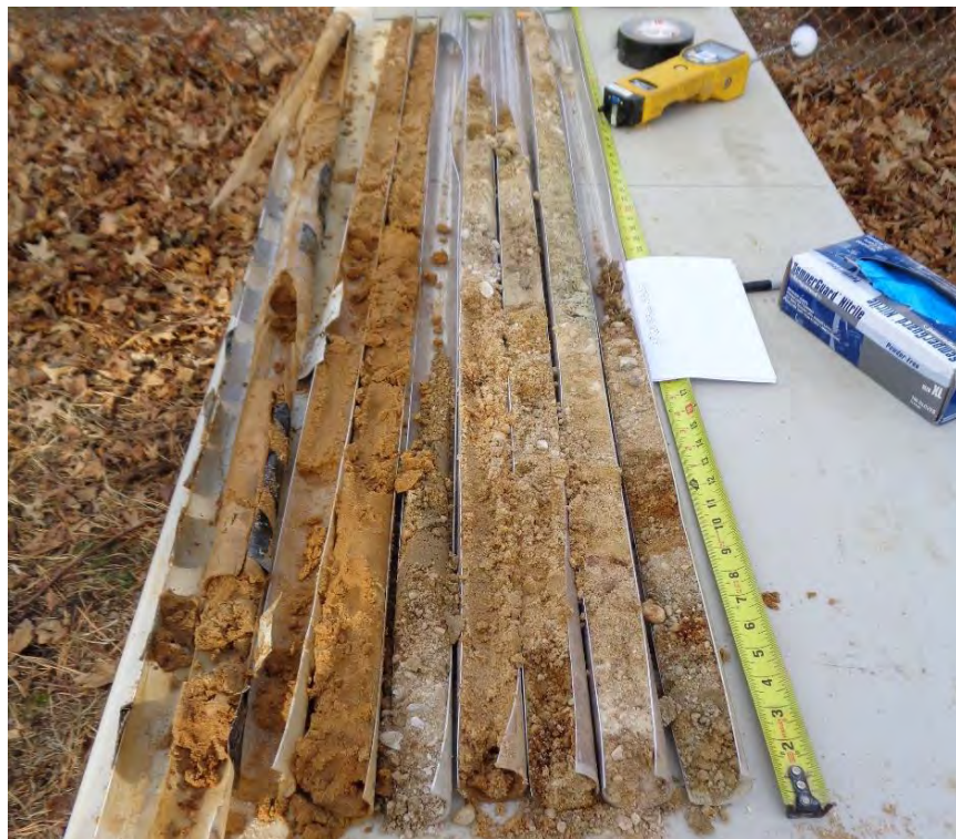
Photo 6: 01/19/2018. Macrocores from soil boring BP-GM38Basin-SB02 from 5 to 40 feet bgs. The first 5 feet were hand augured. The cores are arranged from right to left in descending order.
