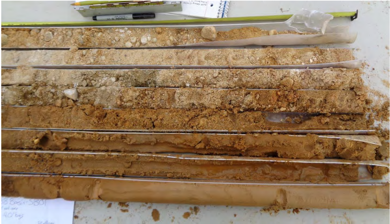
Photo 5: 01/19/2018. Cores are arranged from top to bottom in descending order. Note clay in the bottom two feet of the core from 35 to 40 feet bgs.
