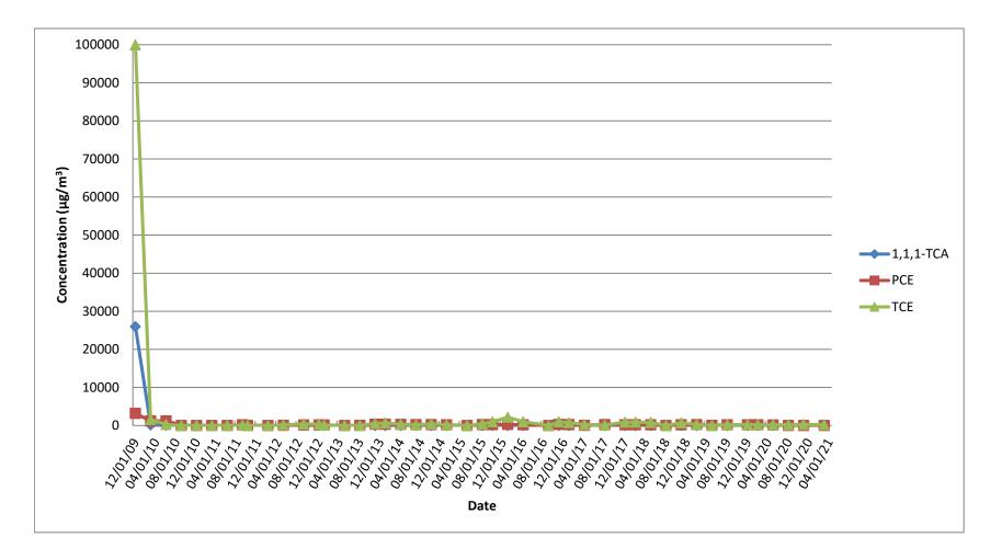
Soil Vapor Extraction Containment System Site 1, Former Drum Marshalling Yard Naval Weapons Industrial Reserve Plant - Bethpage, NY Concentration Trends of Select VOCs SVEWs SV-101D (smaller scale)
