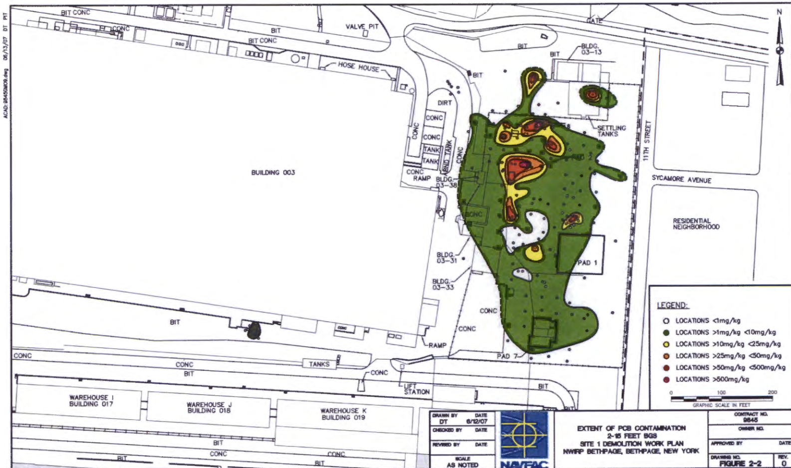
Figure 5. PCB Contamination 2-15 feet Below Ground Surface
