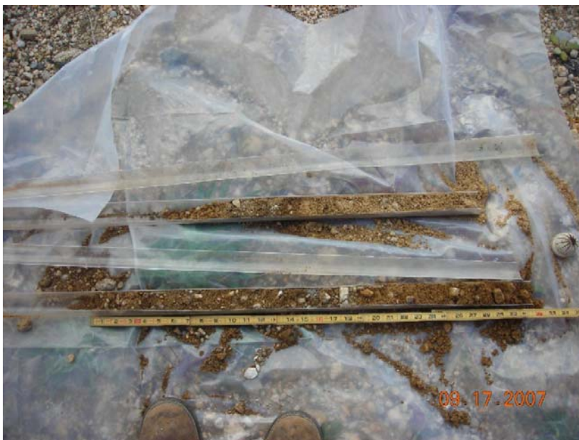
Photo 5 Soil Core from Boring Adjacent to Sampling Location SG-4 Within Former Plant 2 Footprint
