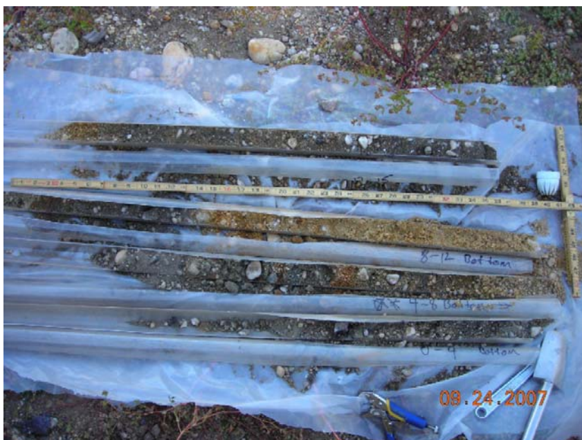
Photo 10 Soil Core from Boring Adjacent to Sampling Location SG-9 West of Former Rainwater Runoff Sump
