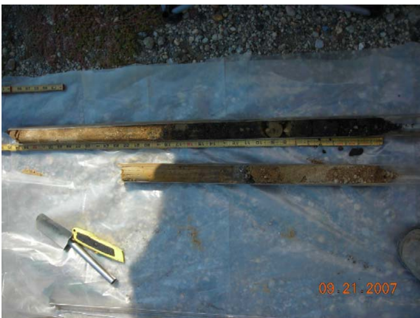
Photo 6 Soil Core from Boring Adjacent to Sampling Location SG-5 West of Former Plant 1 Footprint
