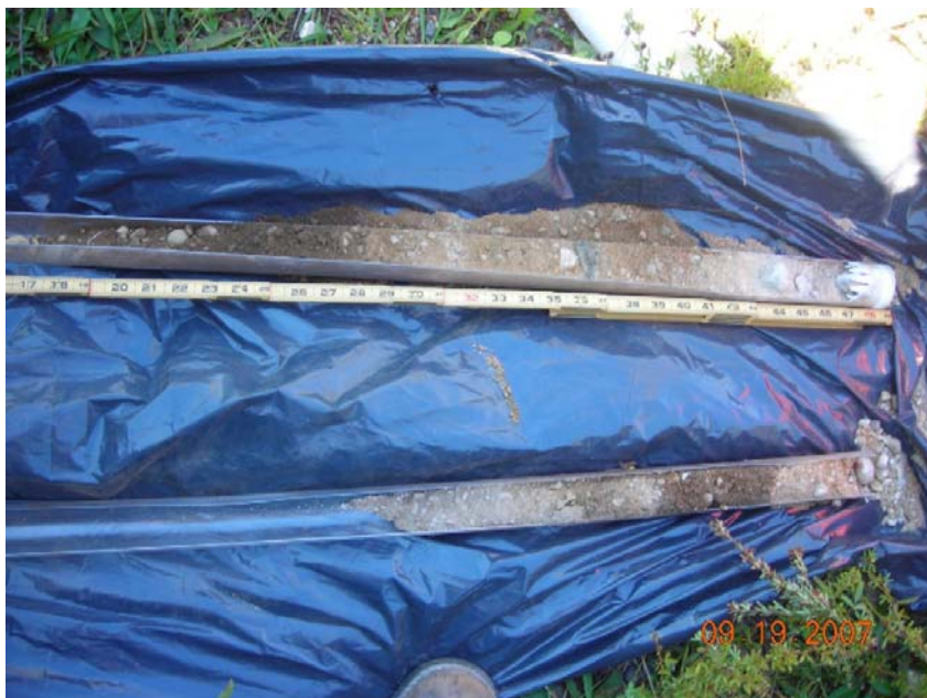
Photo 16 Soil Core from Boring Adjacent to Sampling Location SG-15 Along Eastern Property Boundary
