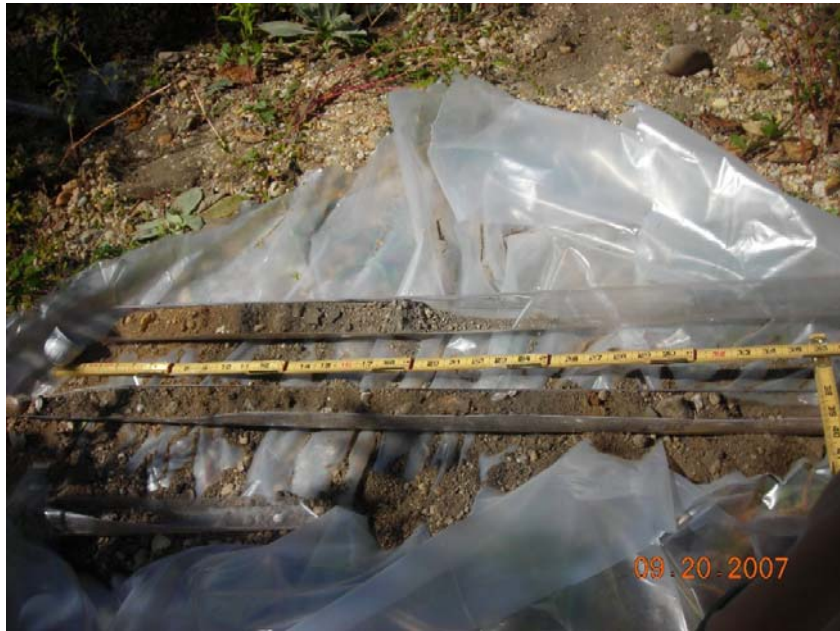
Photo 15 Soil Core from Boring Adjacent to Sampling Location SG-14 Along Eastern Property Boundary
