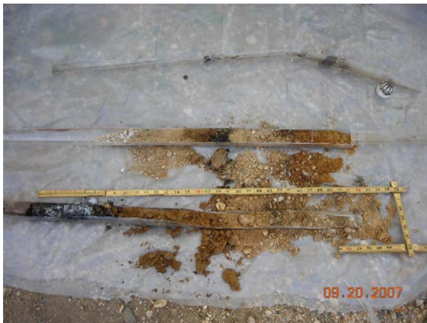
Photo 13 Soil Core from Boring Adjacent to Sampling Location SG-12 Along Southwest Property Boundary
