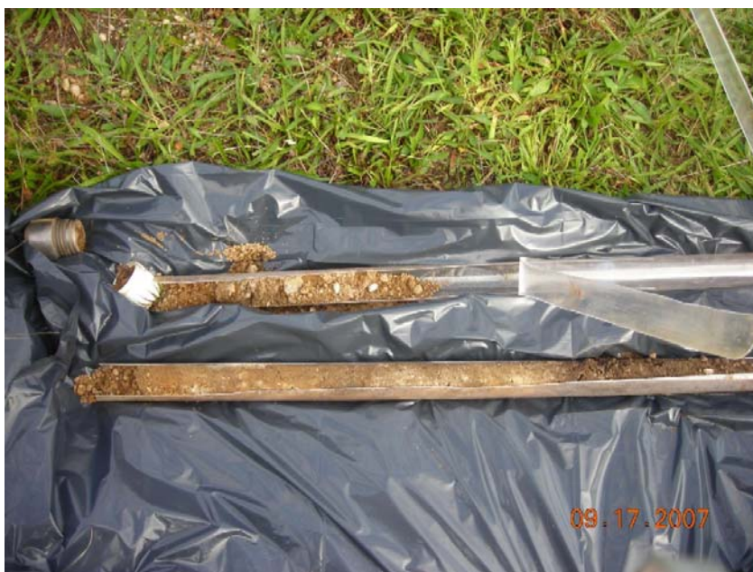
Photo 8 Soil Core from Boring Adjacent to Sampling Location SG-7 North of Former Plant 3 Footprint
