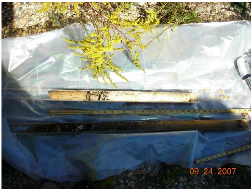
Photo 9 Soil Core from Boring Adjacent to Sampling Location SG-8 Within Former Plant 3 Footprint
