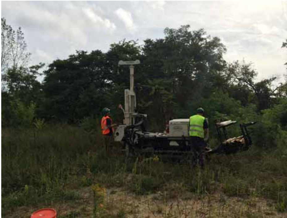
Posillico's drilling subcontractor (Eastern Environmental Inc.) collecting in-situ waste characterization samples.
