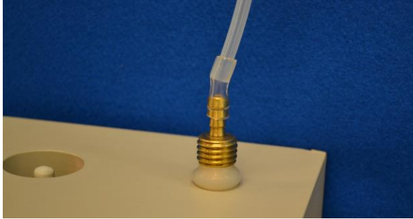
Figure 5. VAPOR PIN® sample connection
