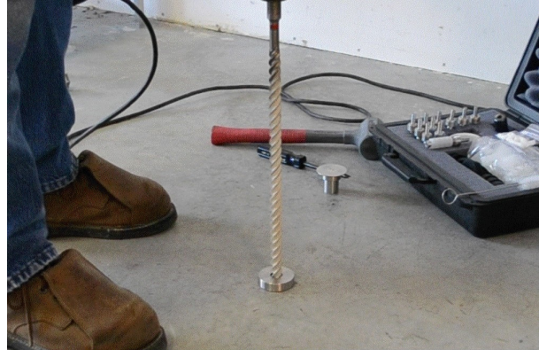
Figure 4. Using the Drilling Guide.
