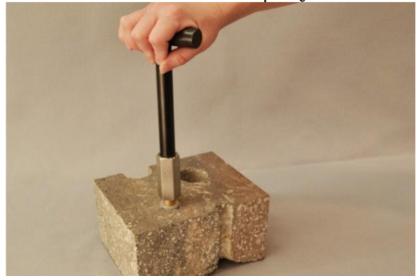
Figure 7. Removing the VAPOR PIN®
