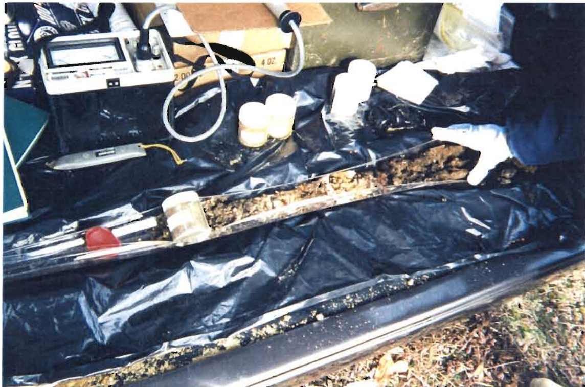
Core of discolored soil from SB-48 at 3 to 8 feet bgs; color ranges from dark grey to grey brown with wood fragments
