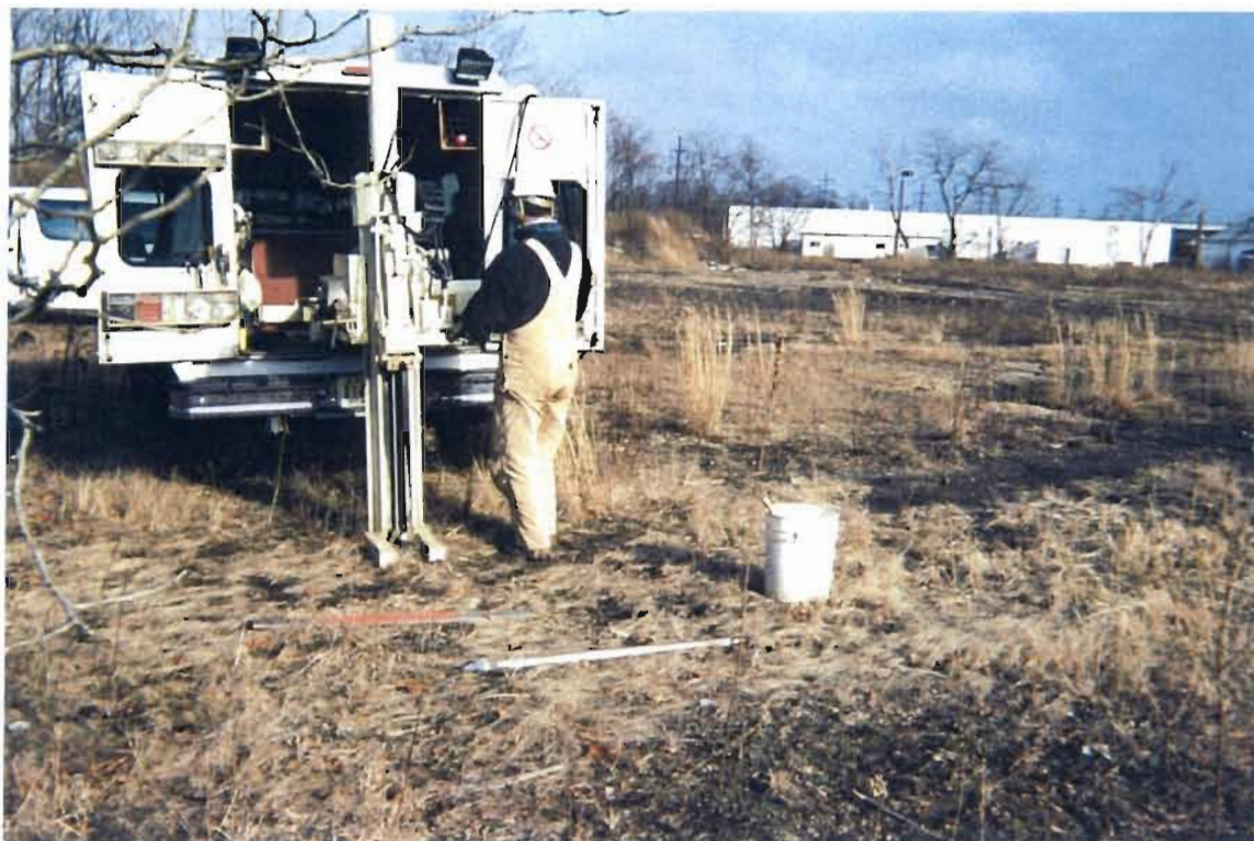
Soil boring location SB-52, showing Geoprobe® drill rig and physical site features
