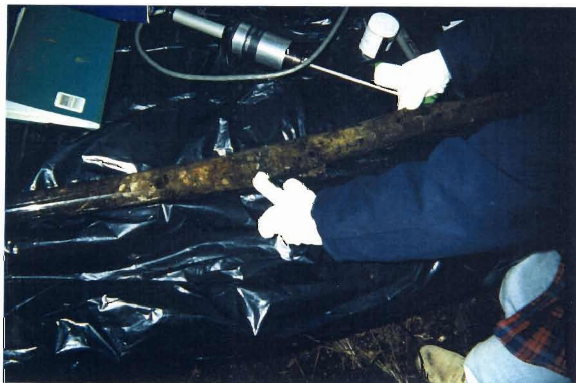
Soil core from SB-44 at 3 to 8 feet bgs; multi-colored fill
