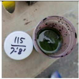
Photo 3: Top view of Oil-In-Soil test on sample collected from 7 to 8 feet bgs at SB-115.
