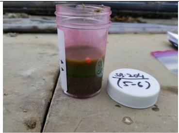
Photo 7: Top view of Oil-In-Soil test on sample collected from 5 to 6 feet bgs at SB-204.
