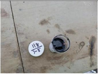
Photo 11: Top view of Oil-In-Soil test on sample collected from 7 to 8 feet bgs at SB-118.
