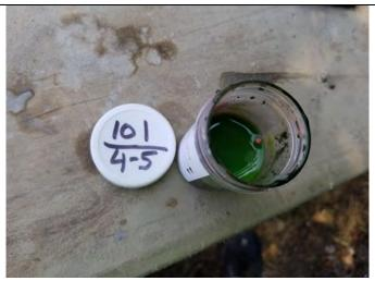
Photo 4: Top view of Oil-In-Soil test on sample collected from 4 to 5 feet bgs at SB-101.
