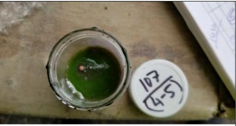
Photo 14: Top view of Oil-In-Soil test on sample collected from 4 to 5 feet bgs at SB-107.
