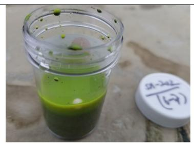
Photo 3: Side view of Oil-In-Soil test on sample collected from 6 to 7 feet bgs at SB-202.
