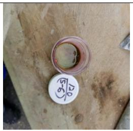
Photo 8: Top view of Oil-In-Soil test on sample collected from 5 to 6 feet bgs at SB-120.
