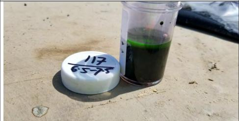
Photo 7: Side view of Oil-In-Soil test on sample collected from 6.5 to 7.5 feet bgs at SB-117.
