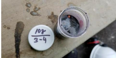
Photo 16: Top view of Oil-In-Soil test on sample collected from 3 to 4 feet bgs at SB-108.
