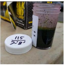
Photo 2: Side view of Oil-In-Soil test on sample collected from 7 to 8 feet bgs at SB-115.
