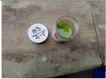
Photo 9: Top view of Oil-In-Soil test on sample collected from 4 to 5 feet bgs at SB-103.
