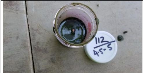
Photo 3: Top view of Oil-In-Soil test on sample collected from 4.5 to 5 feet bgs at SB-112.
