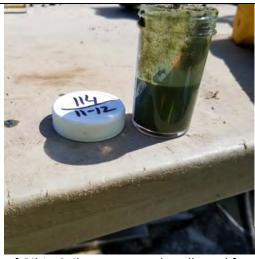
Photo 5: Side view of Oil-In-Soil test on sample collected from 11 to 12 feet bgs at SB-114.
