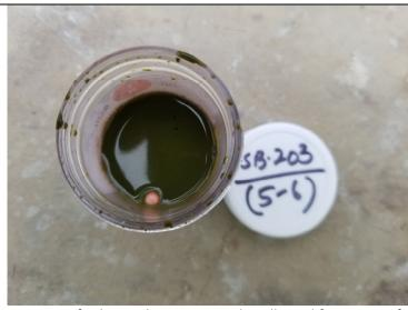
Photo 6: Top view of Oil-In-Soil test on sample collected from 5 to 6 feet bgs at SB-203.
