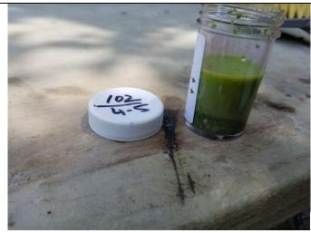
Photo 5: Side view of Oil-In-Soil test on sample collected from 4 to 5 feet bgs at SB-102.
