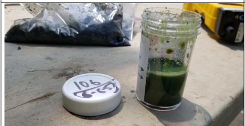
Photo 11: Side view of Oil-In-Soil test on sample collected from 6 to 6.5 feet bgs at SB-106.
