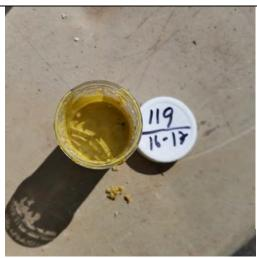
Photo 3: Top view of Oil-In-Soil test on sample collected from 16 to 17 feet bgs at SB-119.
