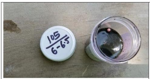
Photo 5: Top view of Oil-In-Soil test on sample collected from 6 to 6.5 feet bgs at SB-105.
