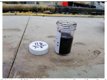
Photo 12: Side view of Oil-In-Soil test on sample collected from 7 to 8 feet bgs at SB-118.
