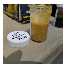
Photo 4: Side view of Oil-In-Soil test on sample collected from 14 feet bgs at SB-115.
