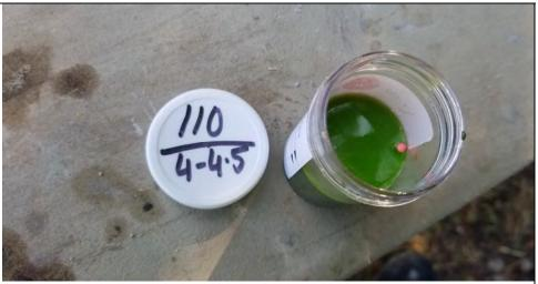
Photo 2: Top view of Oil-In-Soil test on sample collected from 4 to 4.5 feet bgs at SB-110.
