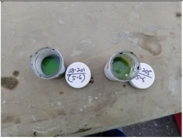
Photo 2: Top view of Oil-In-Soil test on sample collected from 5 to 6 feet bgs at SB-201 and from 5 to 6 feet bgs at SB-205.
