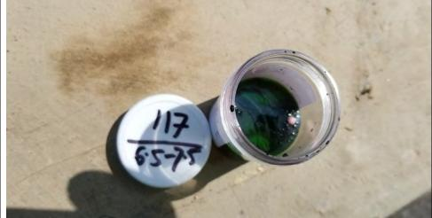
Photo 8: Top view of Oil-In-Soil test on sample collected from 6.5 to 7.5 feet bgs at SB-117.
