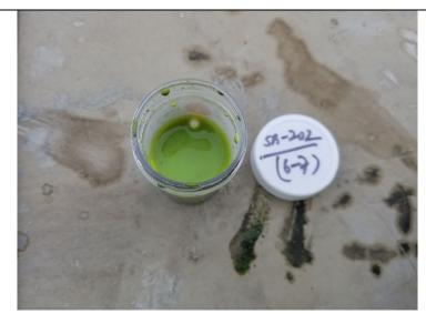
Photo 4: Top view of Oil-In-Soil test on sample collected from 6 to 7 feet bgs at SB-202.
