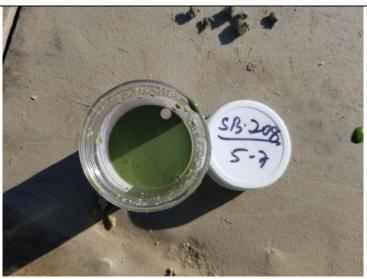
Photo 2: Top view of Oil-In-Soil test on sample collected from 5 to 7 feet bgs at SB-208.
