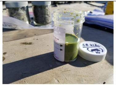
Photo 11: Side view of Oil-In-Soil test on sample collected from 10 bgs at SB-212.
