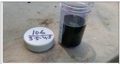
Photo 9: Side view of Oil-In-Soil test on sample collected from 3.5 to 4.5 feet bgs at SB-106.
