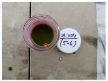
Photo 8: Side view of Oil-In-Soil test on sample collected from 5 to 6 feet bgs at SB-204.
