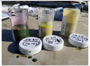
Photo 9: Side view of Oil-In-Soil test on sample collected from 10 to 11 feet bgs, 13 to 14 feet bgs, and 14.5 to 15 feet bgs at SB-211.
