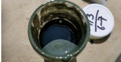
Photo 12: Top view of Oil-In-Soil test on sample collected from 6 to 7 feet bgs at SB-113.
