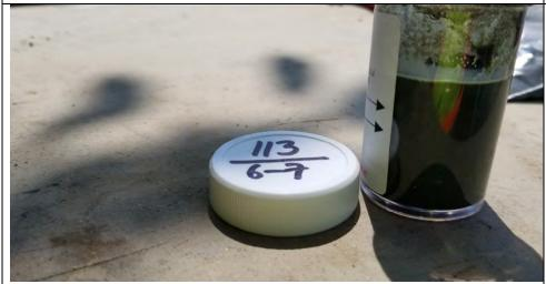
Photo 11: Side view of Oil-In-Soil test on sample collected from 6 to 7 feet bgs at SB-113.
