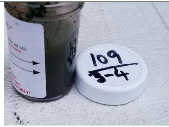
Photo 8: Side view of Oil-In-Soil test on sample collected from 3 to 4 feet bgs at SB-109.
