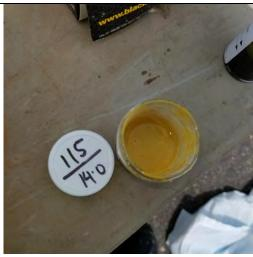
Photo 5: Top view of Oil-In-Soil test on sample collected from 14 feet bgs at SB-115.
