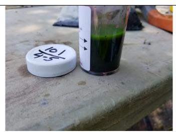
Photo 3: Side view of Oil-In-Soil test on sample collected from 4 to 5 feet bgs at SB-101.
