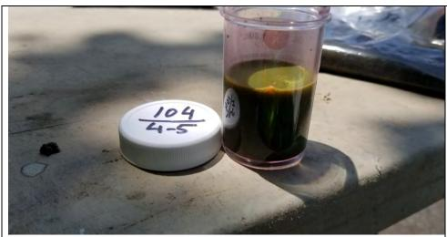
Photo 9: Side view of Oil-In-Soil test on sample collected from 4 to 5 feet bgs at SB-104.
