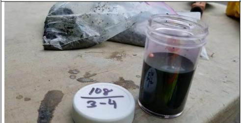
Photo 15: Side view of Oil-In-Soil test on sample collected from 3 to 4 feet bgs at SB-108.
