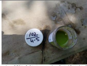
Photo 6: Top view of Oil-In-Soil test on sample collected from 4 to 5 feet bgs at SB-102.
