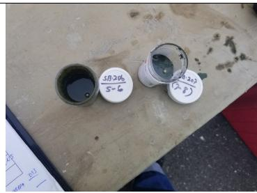
Photo 9: Top view of Oil-In-Soil test on sample collected from 5 to 6 feet bgs at SB-206 and from 7 to 8 feet bgs at SB-207.
