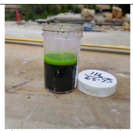
Photo 7: Side view of Oil-In-Soil test on sample collected from 6.5 to 7.5 feet bgs at SB-116.
