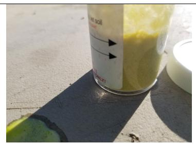
Photo 7: Side view of Oil-In-Soil test on sample collected from 14 to 15 feet bgs at SB-210.
