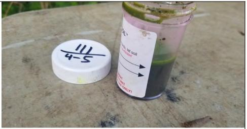
Photo 2: Side view of Oil-In-Soil test on sample collected from 4 to 5 feet bgs at SB-111.
