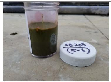
Photo 5: Side view of Oil-In-Soil test on sample collected from 5 to 6 feet bgs at SB-203.
