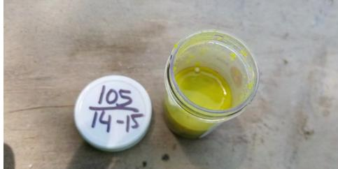
Photo 8: Top view of Oil-In-Soil test on sample collected from 14 to 15 feet bgs at SB-105.
