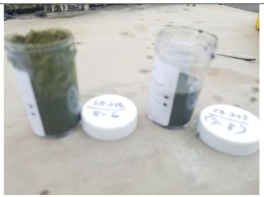
Photo 10: Side view of Oil-In-Soil test on sample collected from 5 to 6 feet bgs at SB-206 and from 7 to 8 feet bgs at SB-207.
