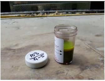
Photo 10: Side view of Oil-In-Soil test on sample collected from 4 to 5 feet bgs at SB-103.
