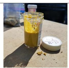
Photo 4: Side view of Oil-In-Soil test on sample collected from 16 to 17 feet bgs at SB-119.
