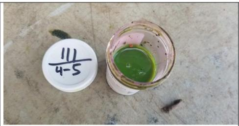
Photo 1: Top view of Oil-In-Soil test on sample collected from 4 to 5 feet bgs at SB-111.
