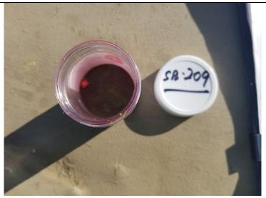
Photo 4: Top view of Oil-In-Soil test on sample collected from 5 to 7 feet bgs at SB-209.
