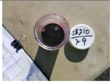
Photo 6: Top view of Oil-In-Soil test on sample collected from 7 to 9 feet bgs at SB-210.
