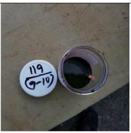
Photo 2: Top view of Oil-In-Soil test on sample collected from 9 to 10 feet bgs at SB-119.
