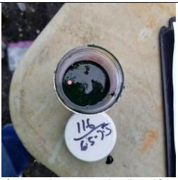
Photo 6: Top view of Oil-In-Soil test on sample collected from 6.5 to 7.5 feet bgs at SB-116.
