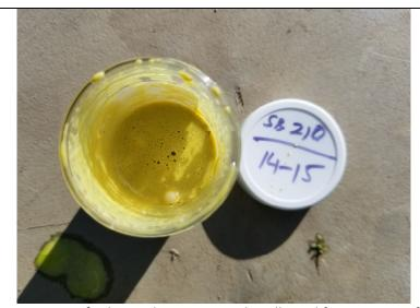
Photo 8: Top view of Oil-In-Soil test on sample collected from 14 to 15 feet bgs at SB-210.
