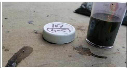
Photo 13: Side view of Oil-In-Soil test on sample collected from 4 to 5 feet bgs at SB-107.
