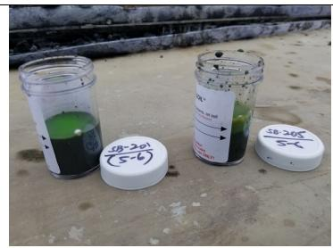
Photo 1: Side view of Oil-In-Soil test on sample collected from 5 to 6 feet bgs at SB-201 and from 5 to 6 feet bgs at SB-205.
