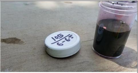
Photo 6: Side view of Oil-In-Soil test on sample collected from 6 to 6.5 feet bgs at SB-105.
