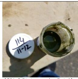
Photo 6: Top view of Oil-In-Soil test on sample collected from 11 to 12 feet bgs at SB-114.
