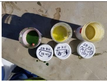
Photo 10: Top view of Oil-In-Soil test on sample collected from 10 to 11 feet bgs, 13 to 14 feet bgs, and 14.5 to 15 feet bgs at SB-211.
