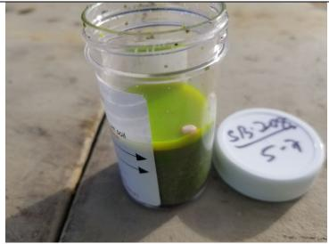
Photo 1: Side view of Oil-In-Soil test on sample collected from 5 to 7 feet bgs at SB-208.
