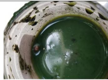
Photo 7: Top view of Oil-In-Soil test on sample collected from 3 to 4 feet bgs at SB-109.
