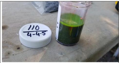
Photo 1: Side view of Oil-In-Soil test on sample collected from 4 to 4.5 feet bgs at SB-110.
