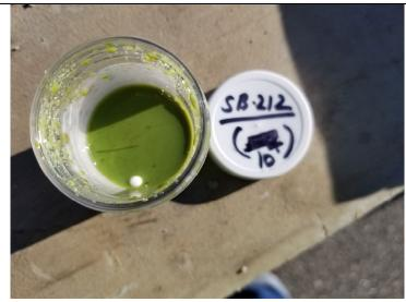
Photo 12: Top view of Oil-In-Soil test on sample collected from 10 feet bgs at SB-212.
