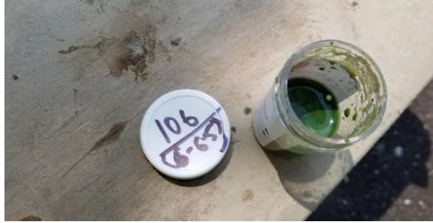
Photo 12: Top view of Oil-In-Soil test on sample collected from 6 to 6.5 feet bgs at SB-106.
