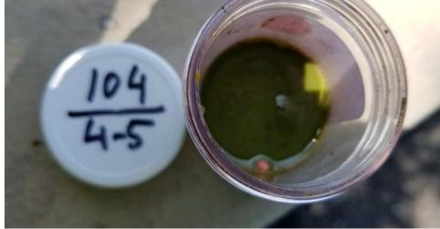
Photo 10: Top view of Oil-In-Soil test on sample collected from 4 to 5 feet bgs at SB-104.
