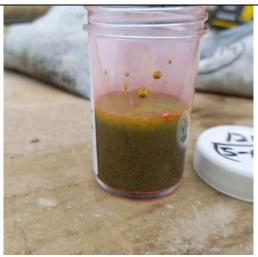
Photo 7: Side view of Oil-In-Soil test on sample collected from 5 to 6 feet bgs at SB-120.
