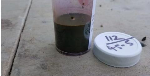
Photo 4: Side view of Oil-In-Soil test on sample collected from 4.5 to 5 feet bgs at SB-112.
