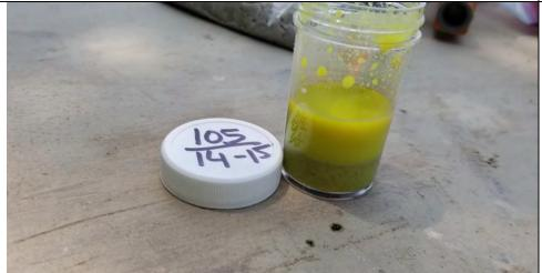
Photo 7: Side view of Oil-In-Soil test on sample collected from 14 to 15 feet bgs at SB-105.
