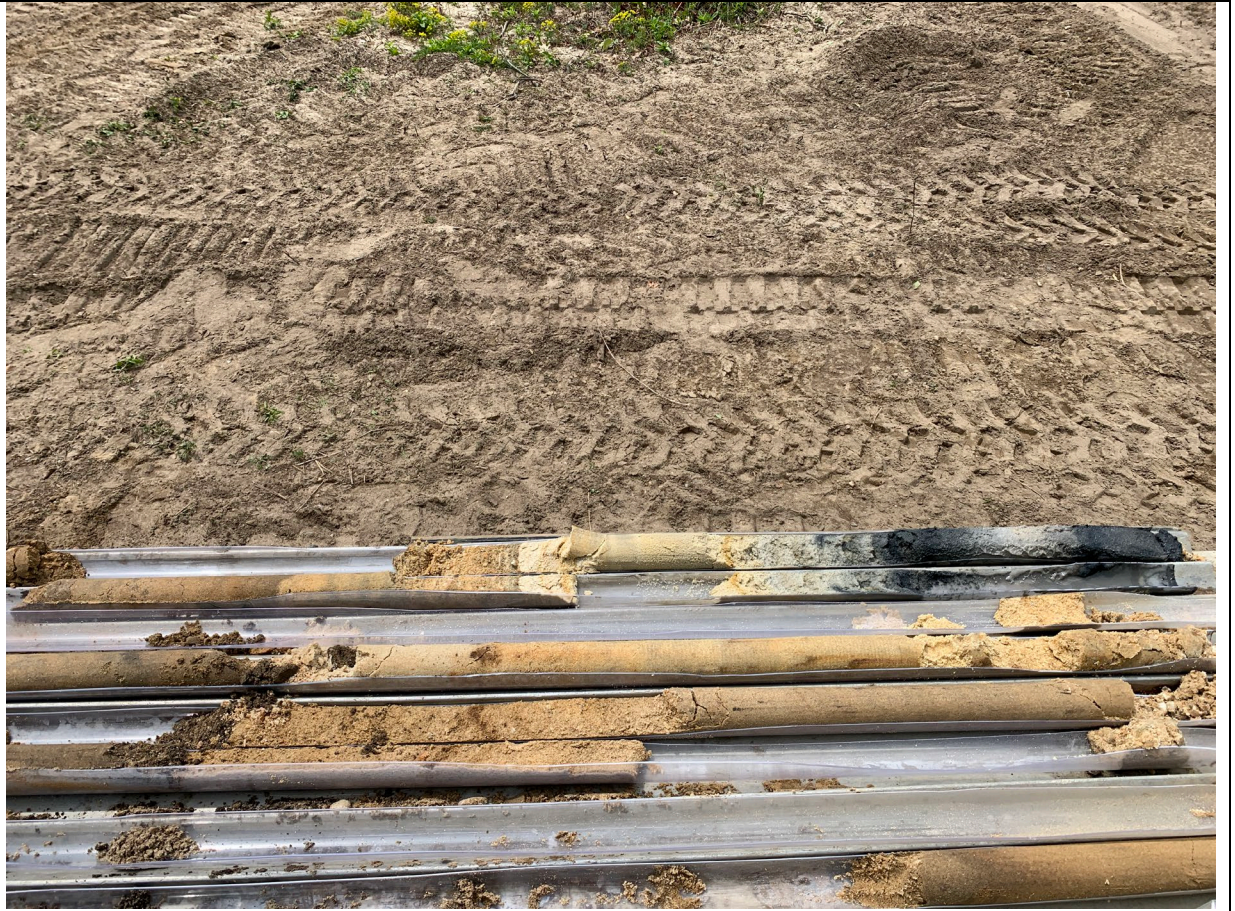
Photo 3 – View of a typical soil boring core, including the darker, impacted soil from the saturated zone.
