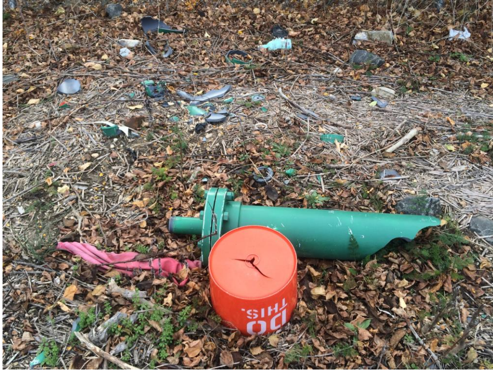
Well Casing Broken at Grade- SW3
