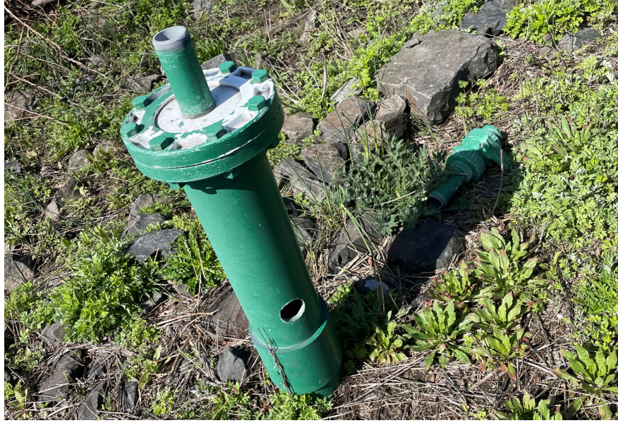
Detached Sampling Assembly – Well SW-7
