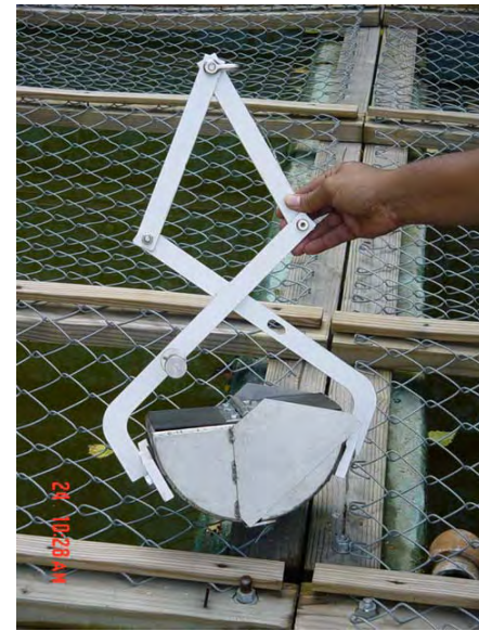
Ponar dredge used to sample storm water pits 7/24/2003
