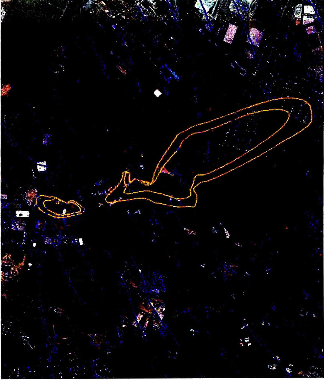
Figure 3-4. USGS MODFLOW/MT3D Predicted TCE Plume in 5 years for Zone A TCE Plume Map Contour Interval = 5, 10, and 50 ug/L
