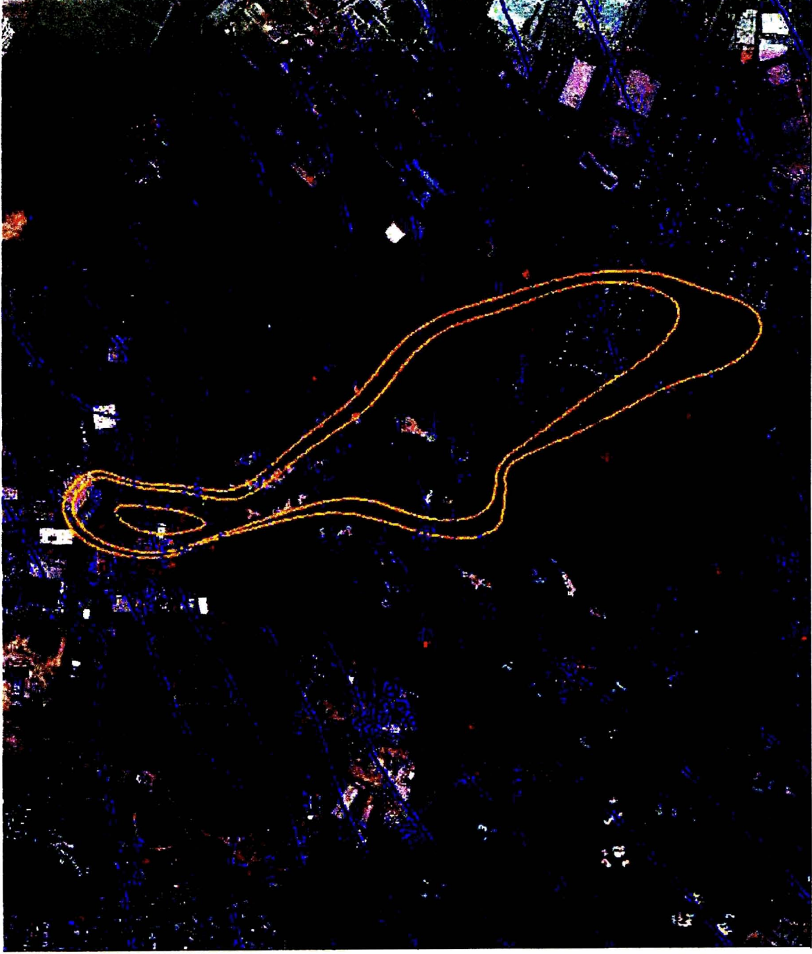
Figure 3-6. USGS MODFLOW/MT3D Predicted TCE Plume in 5 Years for Zone C TCE plume map contour interval = 5, 10, and 50 ug/L
