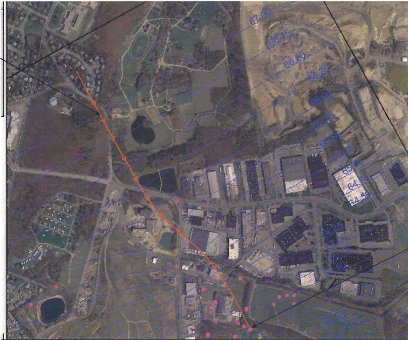
Backward Particle Tracking at Zone C from Well EW-2D (County injection wells, County infiltration pond, Claremont injection wells, and Claremont pumping wells turned off)
