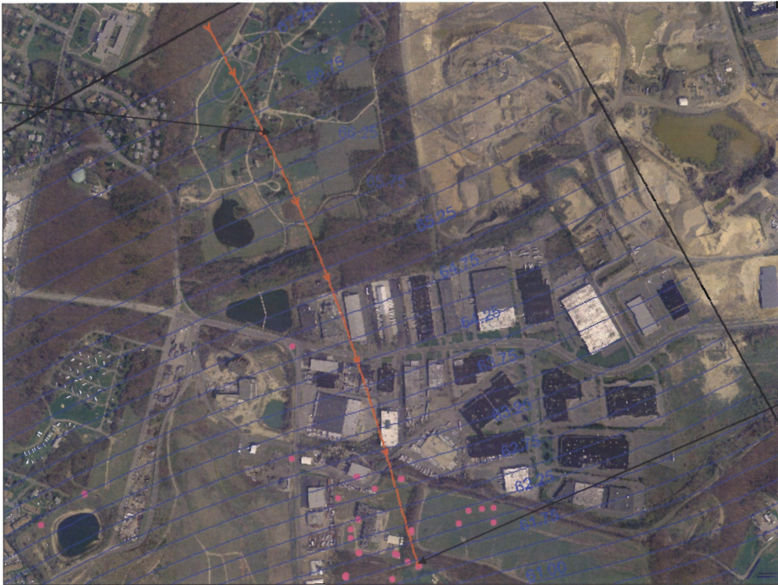
Backward Particle Tracking at Zone C from Well EW-2D (TOB infiltration basins, County injection wells, County infiltration pond, Claremont injection wells, and Claremont pumping wells turned off)
