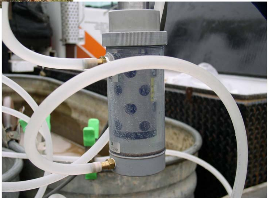
Degassing of purge water during ground water sampling At EW-13D (Horiba U-22 and Flow through cell)
