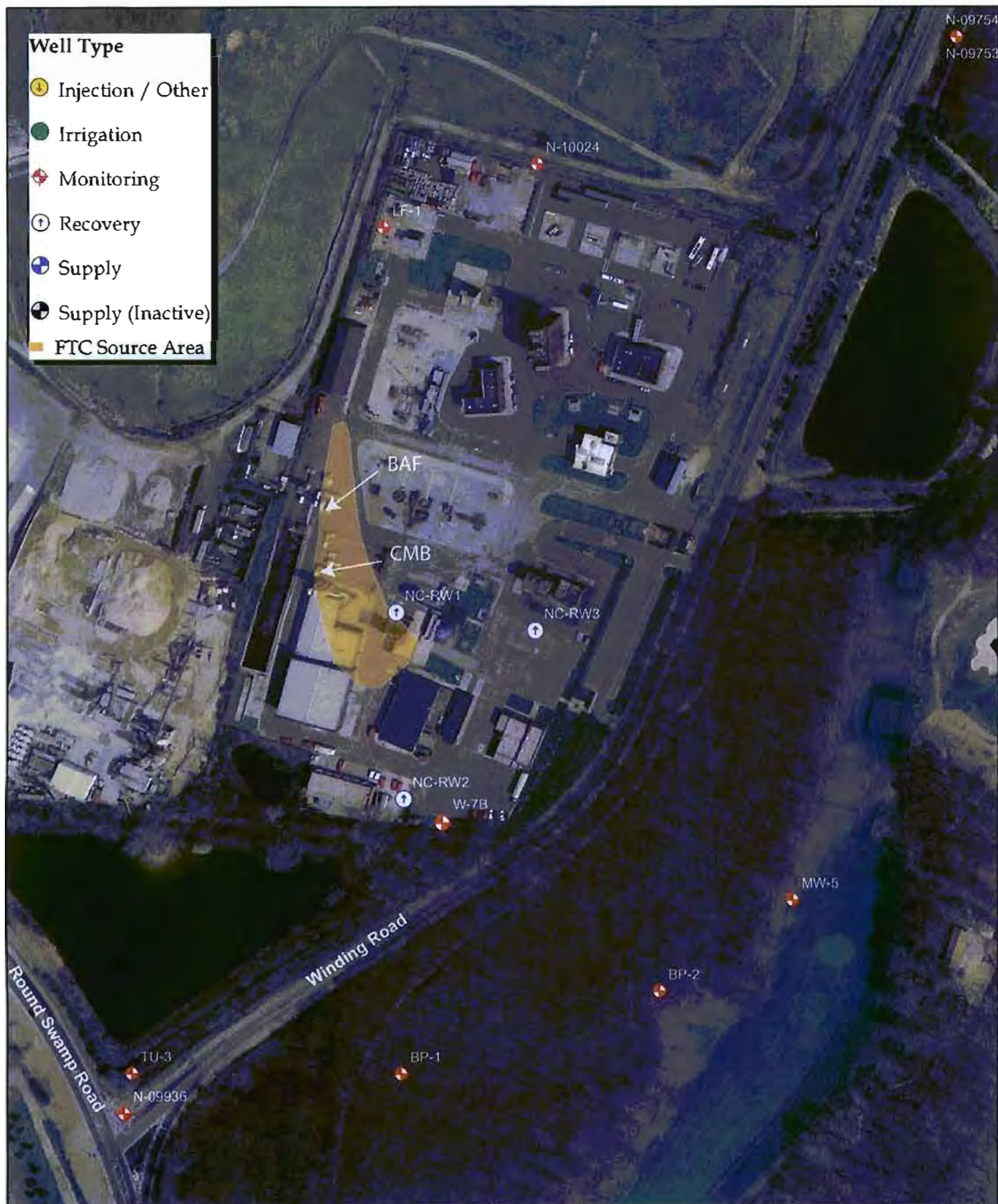
Figure 3-2 Firemen's Training Center Groundwater Model Source Area for Contamination at FTC Facility
