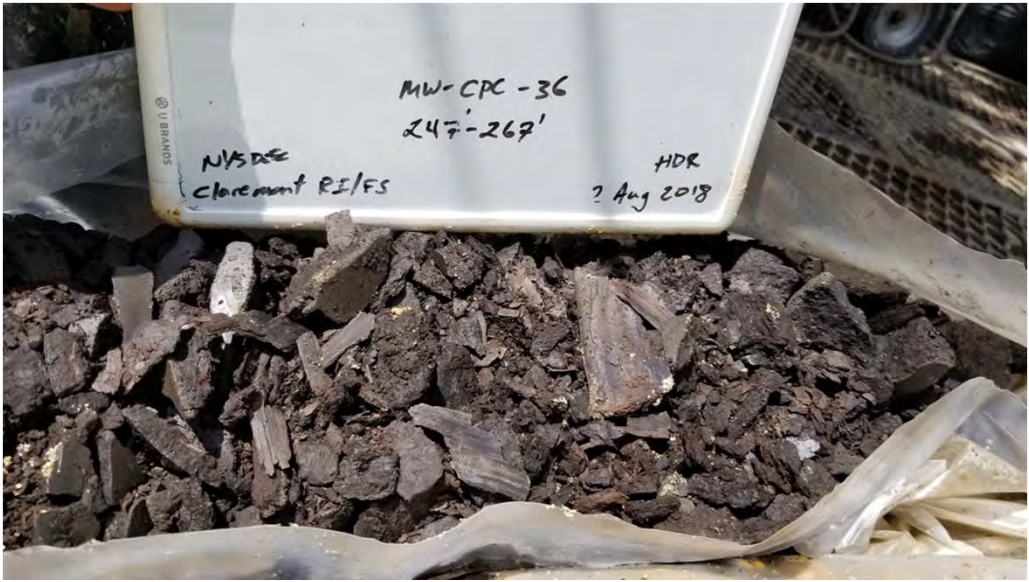
Soil boring MW-CPC-36 – lignite in clay unit
