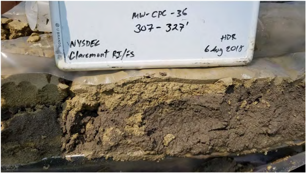
Soil boring MW-CPC-36 – tan-brown mottled fine-coarse sand
