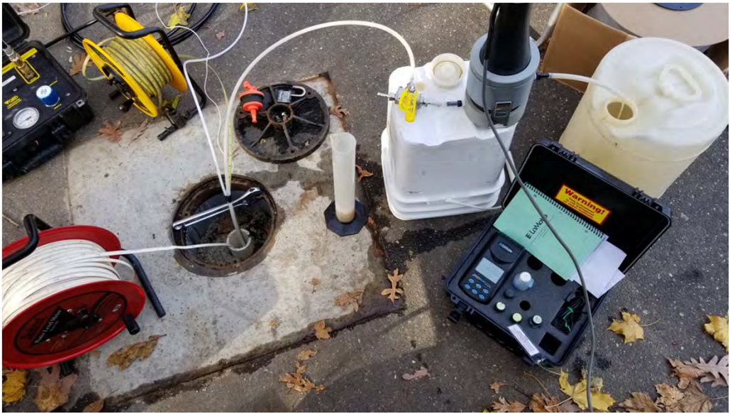
Low flow sampling to collect samples at four boring locations.
