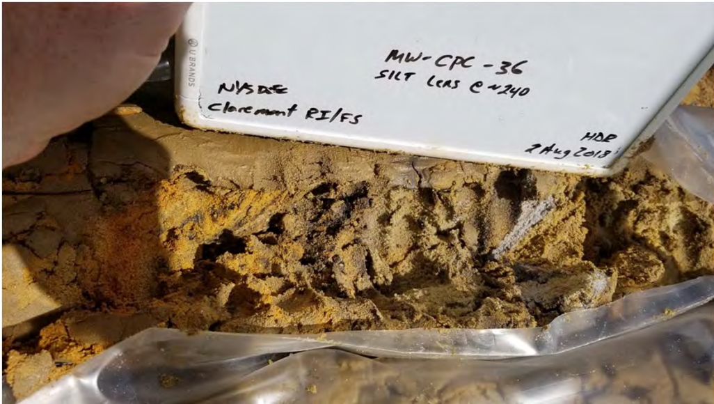
Soil boring MW-CPC-36 – silt lenses in sand matrix
