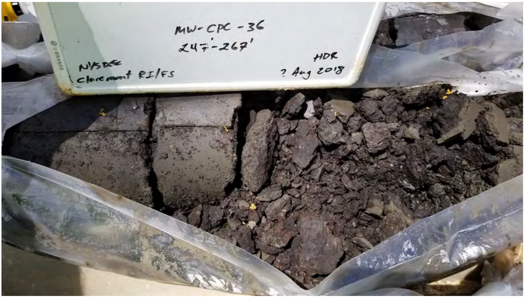
Soil boring MW-CPC-36 – dark gray very stiff dry clay
