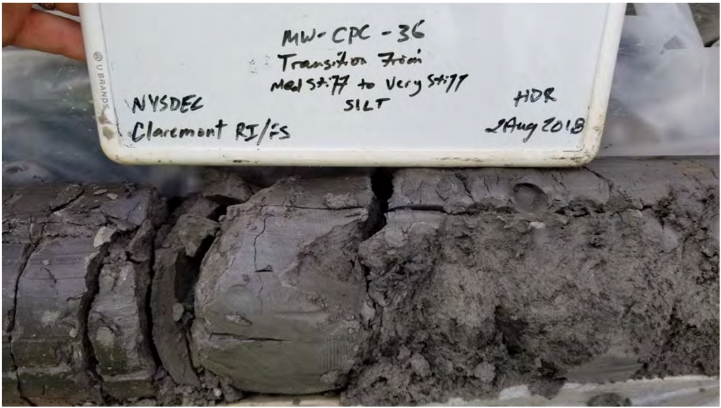
Soil boring MW-CPC-36 – gray moist silty clay unit
