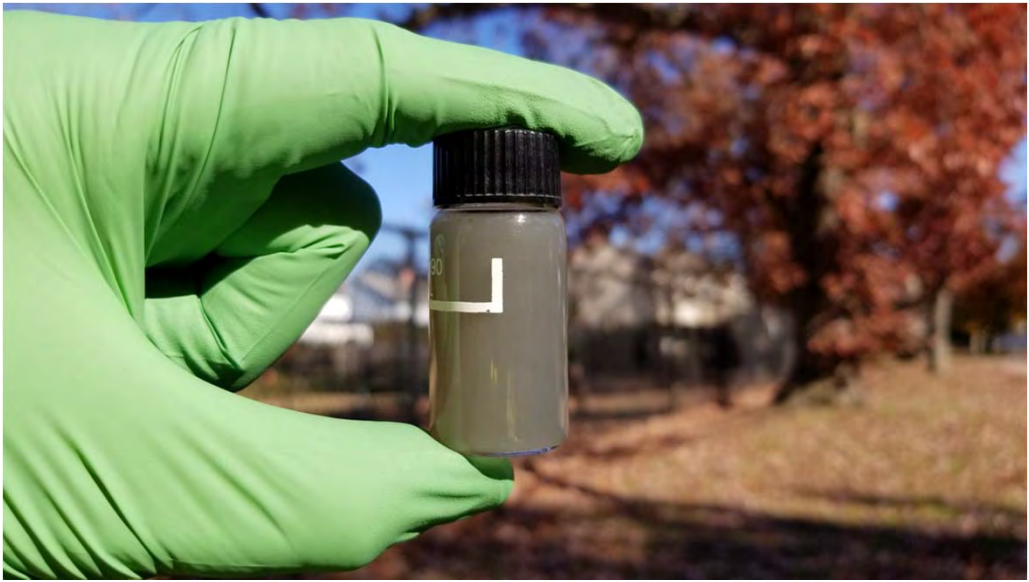
HDR collects turbidity measurements throughout well development process.
