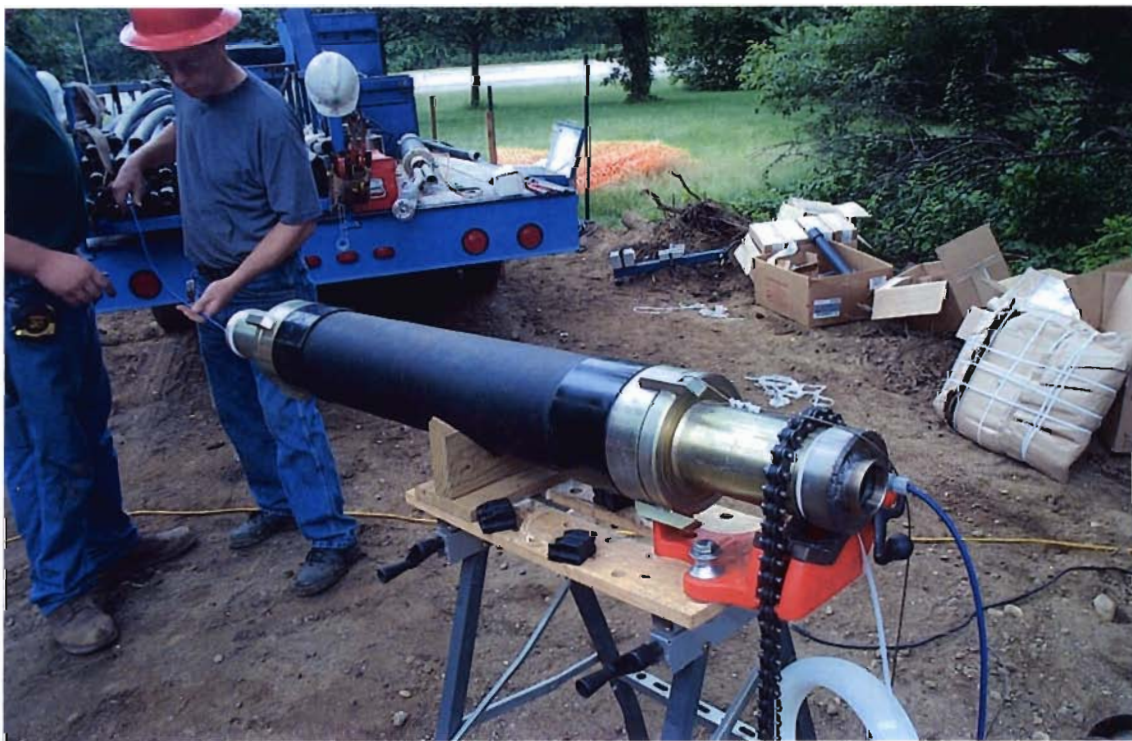
Photograph 7: Threading transducer cables through the packers.
