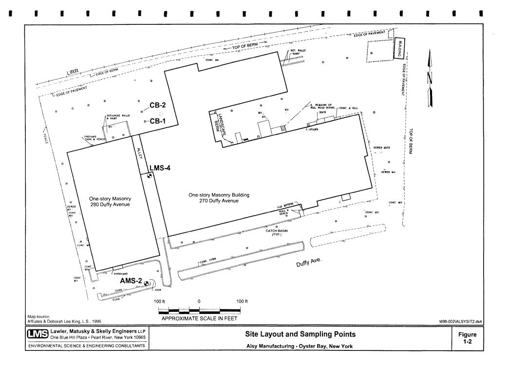
Soil samples were collected from test borings installed using a truck mounted drill rig equipped with hollow stem augers. Each soil sample was removed using a 2-ft split spoon driven ahead of the augers. Samples began at the sediment surface and continued to the water table in 10 ft intervals (approximately 60-ft below grade). Samples from each location were collected from 20 to 22-ft, 30 to 32-ft, 40 to 42-ft, 50 to 52-ft, and 60 to 62-ft.
