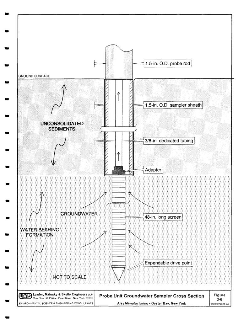
check ball was repeatedly raised and lowered. Groundwater samples were transferred from the tubing directly into laboratory-cleaned bottles and labeled with the appropriate sample location, interval, date, time, sampler, and analyses required. The samples were logged on the appropriate chain-of-custody form and either hand delivered or delivered via courier to the analytical laboratory.
