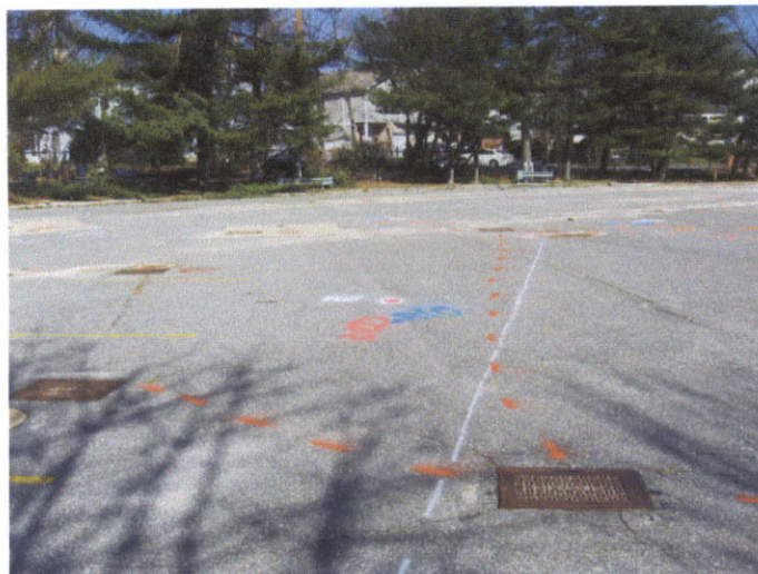
Photograph 10: View looking north toward R-SB-10. Electric lines are visible extending between the electric vaults and a small metal anomaly is visible immediately south of the PEBS.
