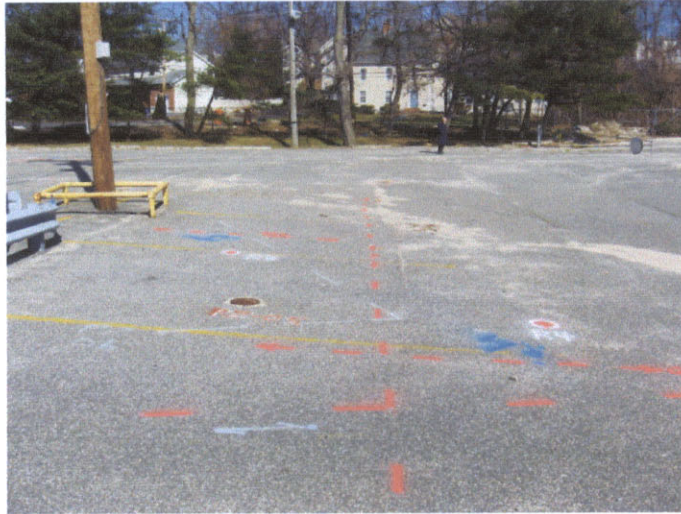
Photograph 3: View looking north toward PEBS R-SB-3 and R-SB-4. A suspected utility is visible in a north to south orientation. A second suspected utility and a linear GPR anomaly are visible in an east-west orientation.
