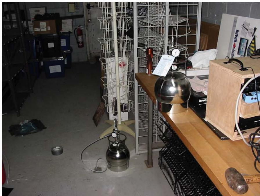
Sampling Structure 7 Sub-Slab and Indoor Air
