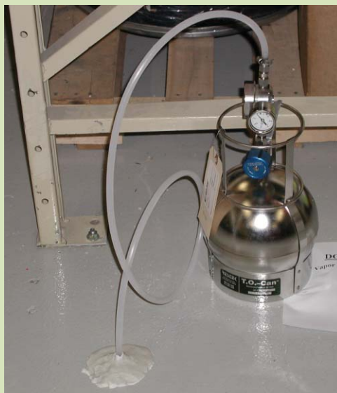
Sub-slab sample point (above), small hole drilled into concrete, patched after sample collection. Indoor air sample point (right)
