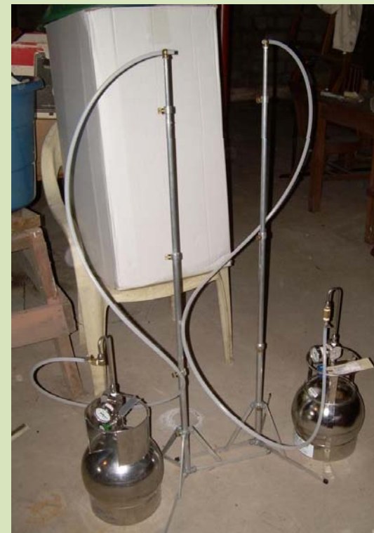
Sub-slab sample point (above), small hole drilled into concrete, patched after sample collection. Indoor air sample point (right)
