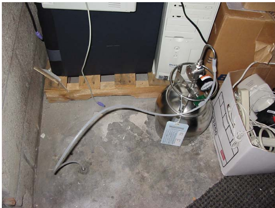
Sampling Structure 7 Sub-Slab
