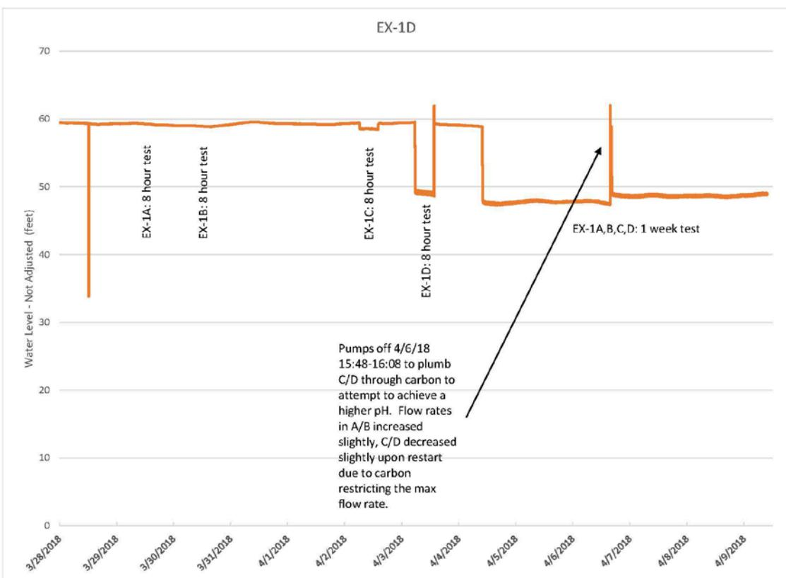
The graphs below present a summary of the system operational data (flow rates and total volume extraction) during Phase I of the pump test.
