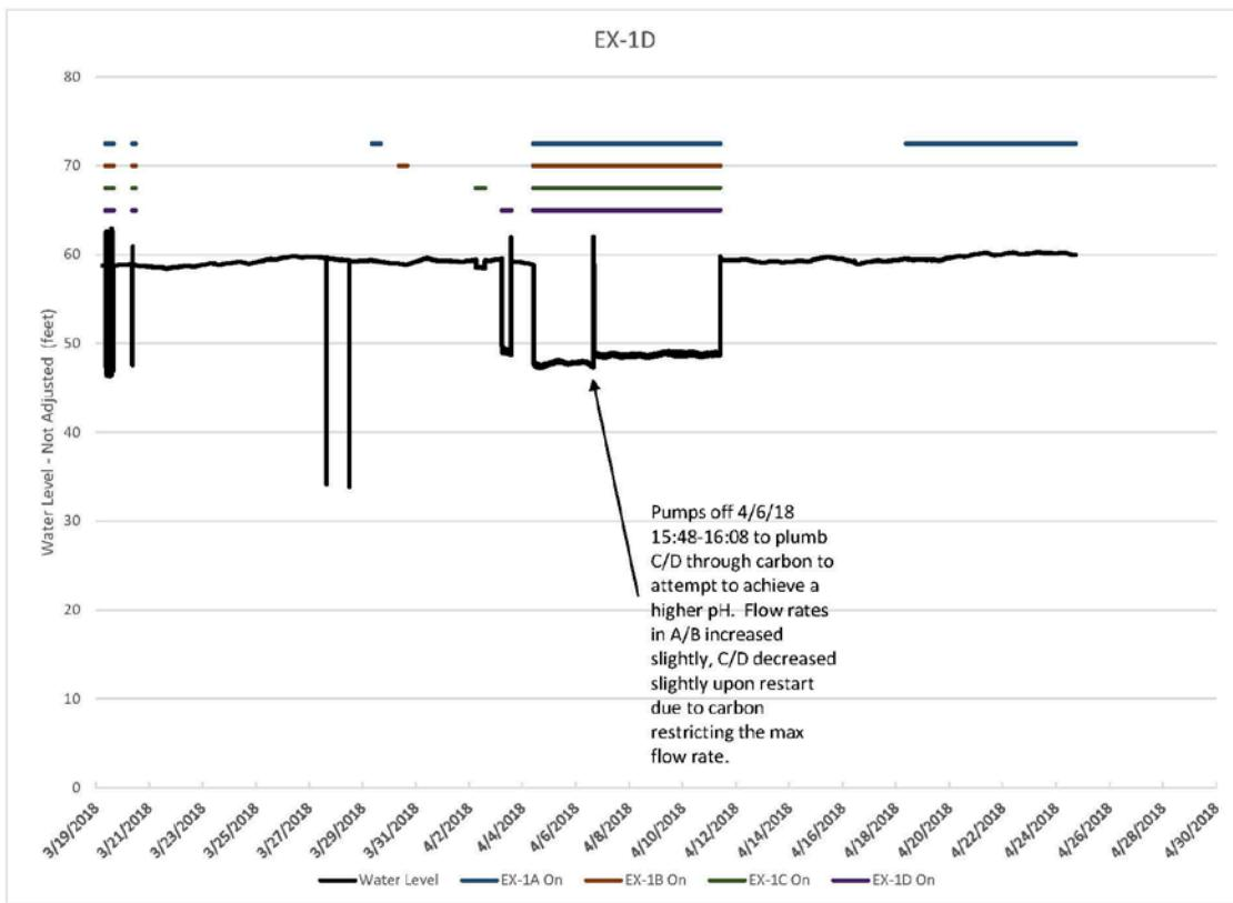
The graphs below present a summary of the system operational data (flow rates and total volume extraction) during the pump test to date (including Phase I of the test).
