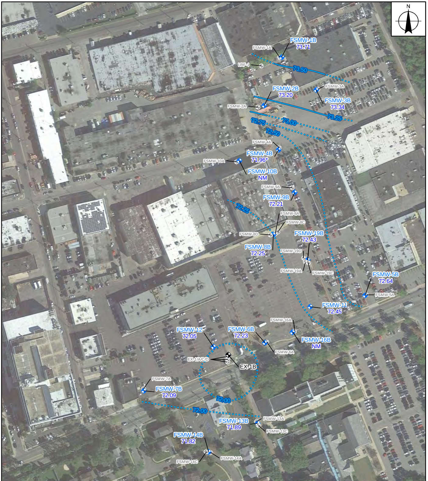
FIGURE 6 POTENTIOMETRIC SURFACE MAP GROUP B WELLS (114-149 FEET BGS) EX-1B AT 33 GPM FROST STREET SITES WESTBURY, NEW YORK
