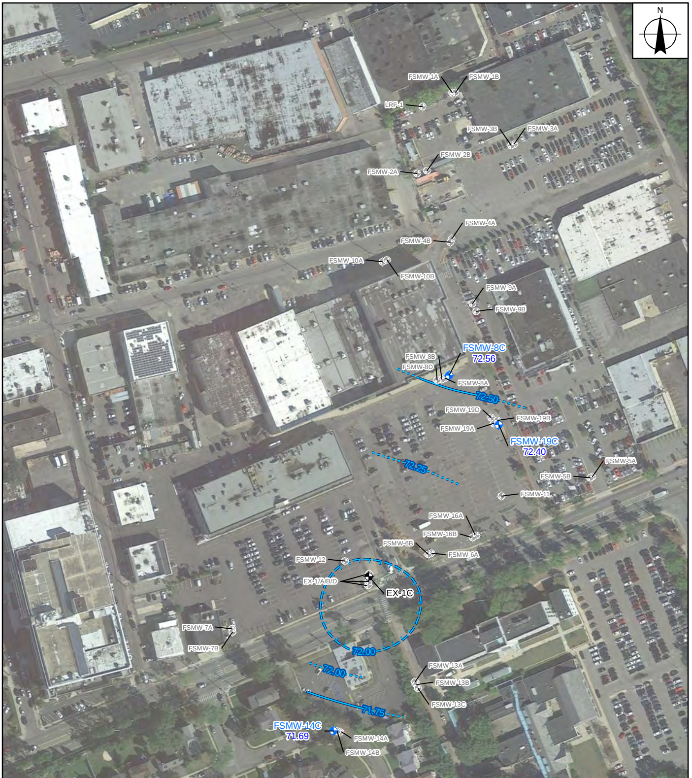
FIGURE 7 POTENTIOMETRIC SURFACE MAP GROUP C WELLS (150-200 FEET BGS) EX-1C AT 44 GPM FROST STREET SITES WESTBURY, NEW YORK
