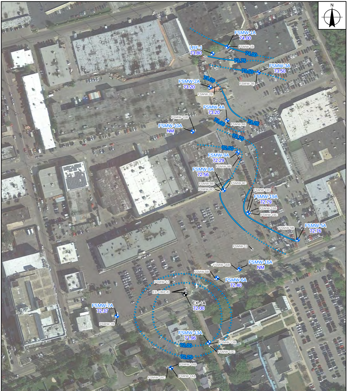
FIGURE 5 POTENTIOMETRIC SURFACE MAP GROUP A WELLS (58-74 FEET BGS) EX-1A AT 33 GPM FROST STREET SITES WESTBURY, NEW YORK
