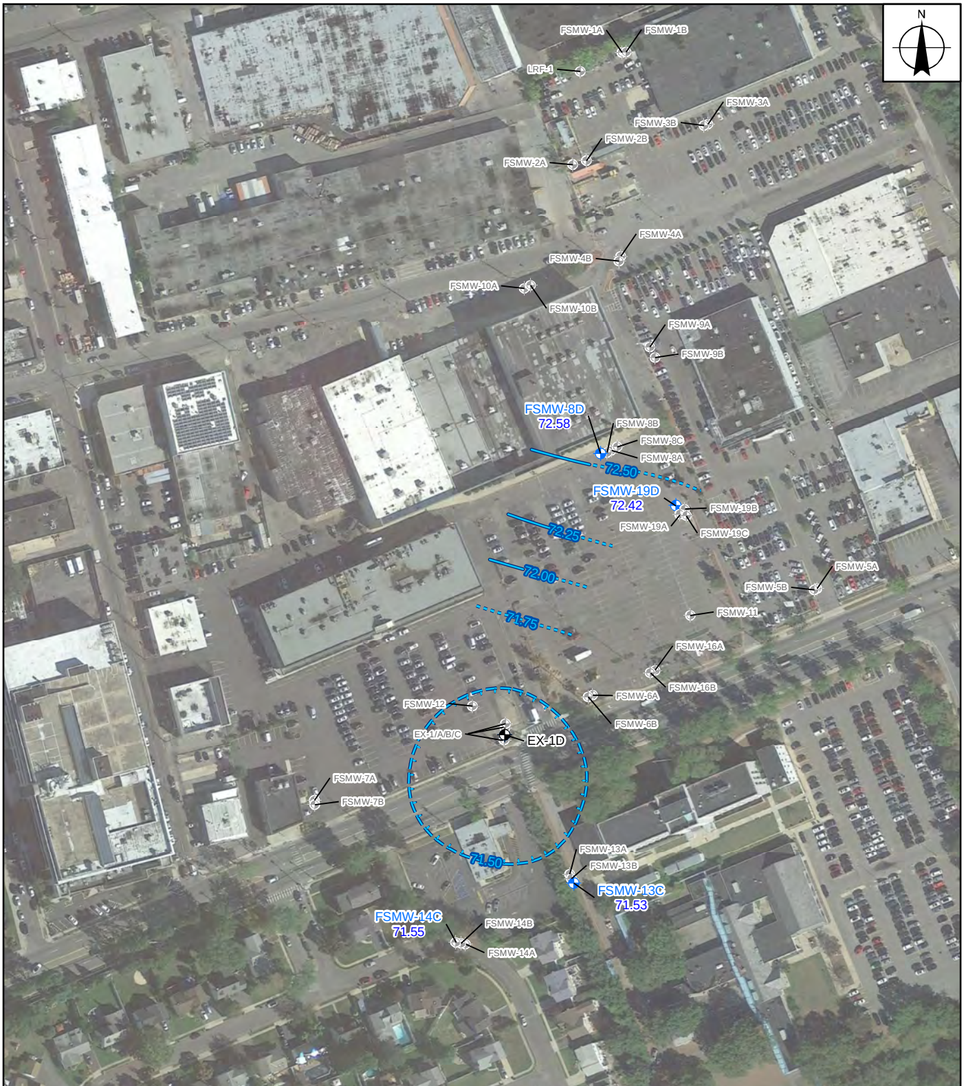
FIGURE 8 POTENTIOMETRIC SURFACE MAP GROUP D WELLS (200-249 FEET BGS) EX-1D AT 44 GPM FROST STREET SITES WESTBURY, NEW YORK
