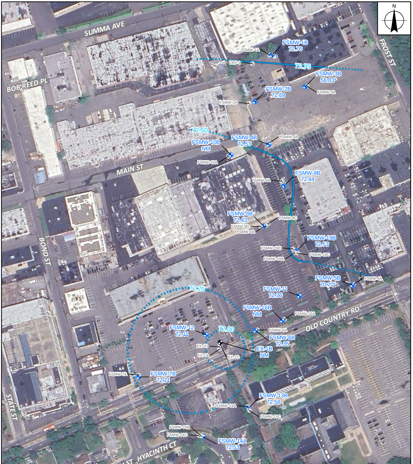
FIGURE 6 POTENTIOMETRIC SURFACE MAP GROUP B WELLS (114-149 FEET BGS) EX-1B AT 30 GPM THIRD QUARTER 2023 FROST STREET SITES WESTBURY, NEW YORK
