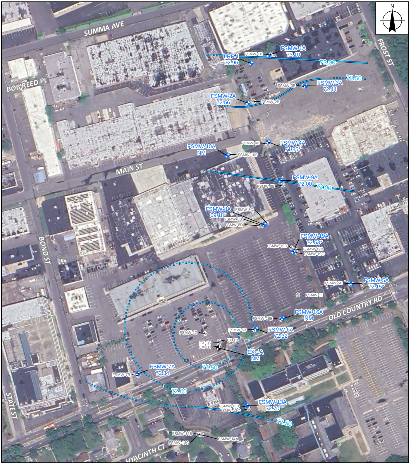
FIGURE 5 POTENTIOMETRIC SURFACE MAP GROUP A WELLS (58-74 FEET BGS) EX-1A AT 33 GPM THIRD QUARTER 2023 FROST STREET SITES WESTBURY, NEW YORK
