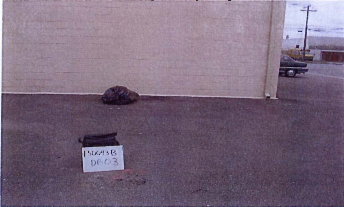
Point DP-03 at side of building for soil vapor and groundwater on Site B
